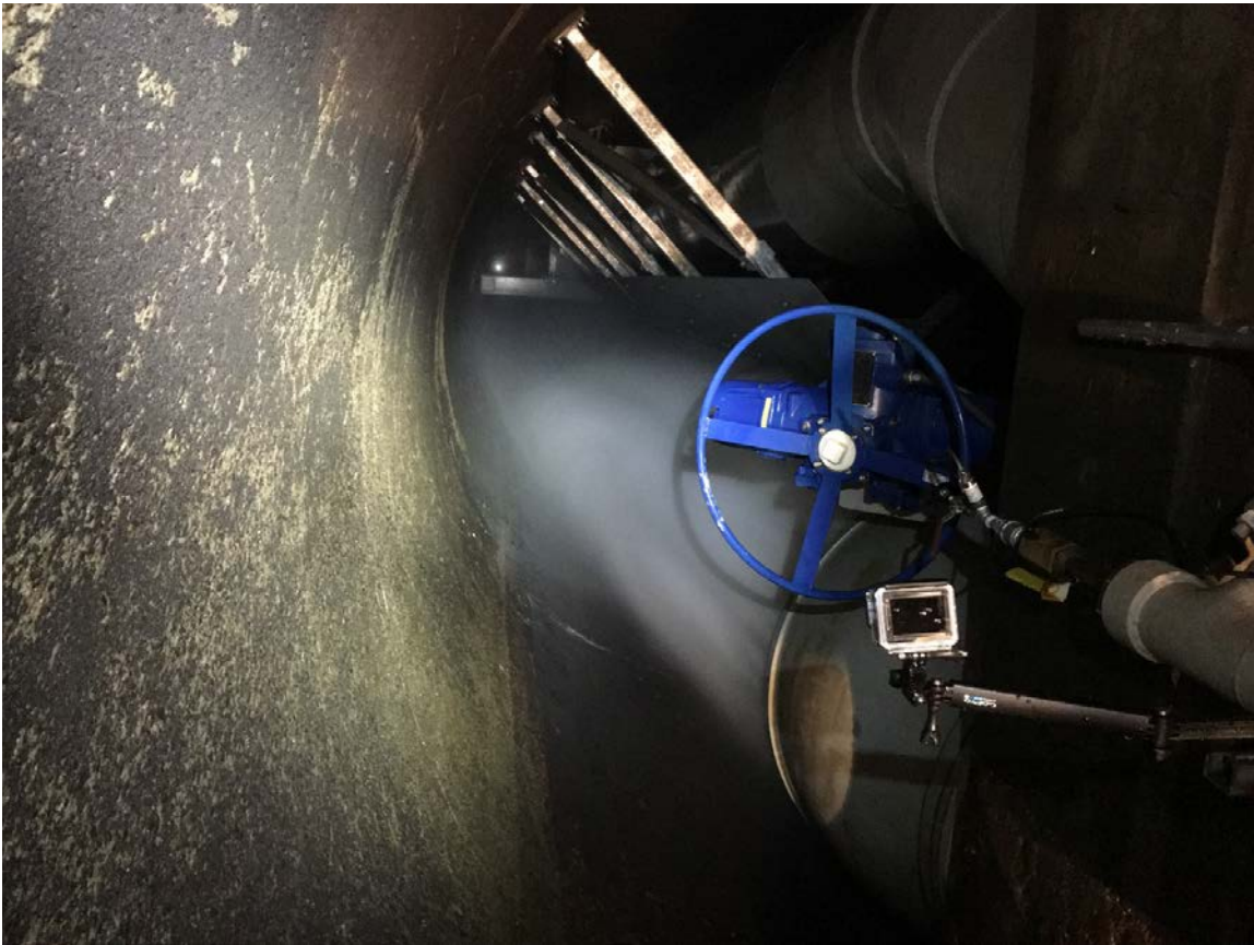
Figure 9 Flow discharging from the hollow jet valve into the tunnel at 50 percent open (about 220 ft 3 /s).
