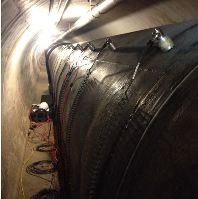
Figure 1. - Accelerometers mounted using magnetic bases (view looking upstream).
