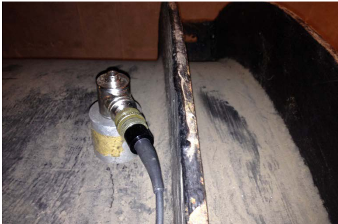
Figure 2. Accelerometer #1 located just upstream of downstream-most ring support.
