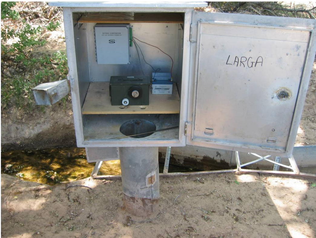
Figure 4—Sutron 8210 datalogger with shaft encoder.
