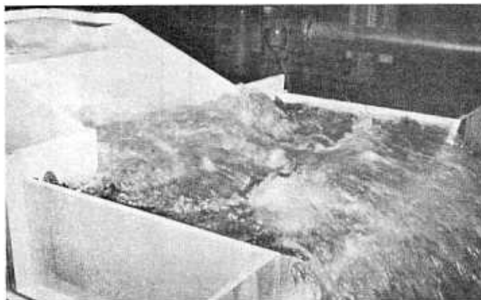
Figure 16.—Entrance pipe flowing full with controlled tailwater in 2.4-foot (730-mm) wide basin.
