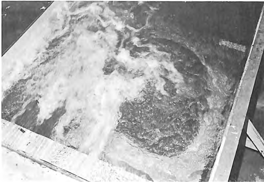
A. Large eddy, reservoir elevation 6769.0, tailwater elevation 6732.0. Photo P17-D-66276
