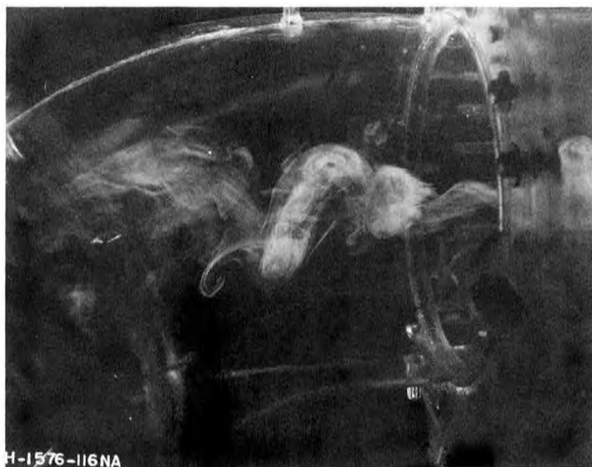
B. Fully established surging in the model of the Fontenelle Draft Tube.
