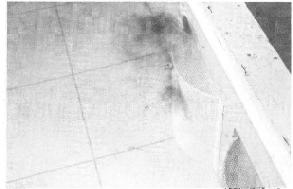
d. Vortex dissipated with some remaining circulation passing over the trashrack. Photo P1222-D-76676
