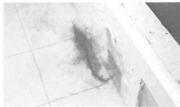
c. Vortex which developed from a swirl. Photo P1222-D-76658
