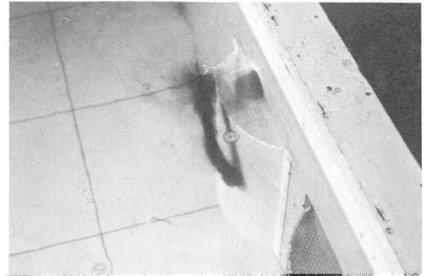
b. Vortex has moved closer, trashrack face resists vortex core circulation. Because of friction, the circulation speed has reduced and the vortex core widens. Photo P1222-D-76674
