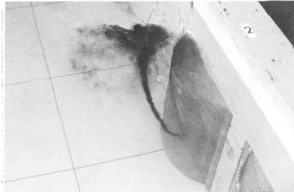
a. Well-developed vortex with a small core of rapidly circulating water. Photo P1222-D-76673
