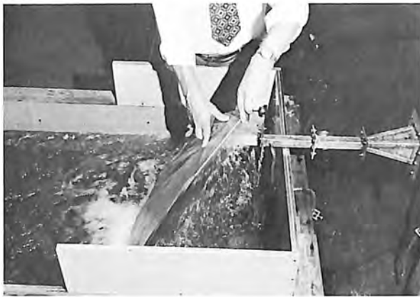
Figure 2. Shield to spread and deflect the jet away from the scour test area.
