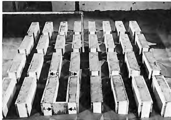
Figure 15. Test 10. Backfill material pumped into a dry cavity. Note deposit in corridor that is blocked. Slurry concentration was 20 percent. Photo P801-D-73851
