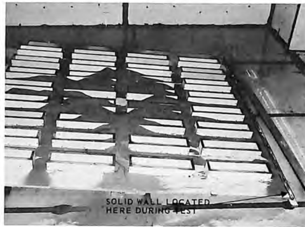
Figure 25. Test 17. The floor and roof of the mine cavity was sloping 5^{\circ} from the horizontal. A solid wall was simulated at the downslope end of the pillars. Photo P801-D-73858
