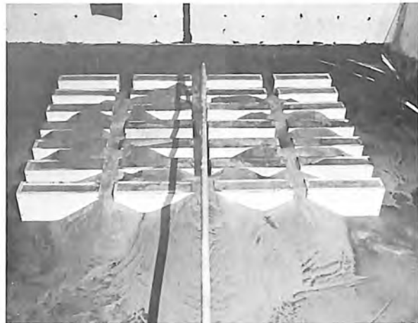
Figure 7. Test 6. Deposit pattern after injection of 16 percent backfill material at a pipe injection velocity of 15 feet per second. Photo P801-D-73845
