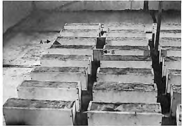
Figure 14. Test 10. Arrangement of pillars for backfill material pumped into a dry cavity. Blocks in one corridor were placed at A, B, and C as shown. Photo P801-D-73849
