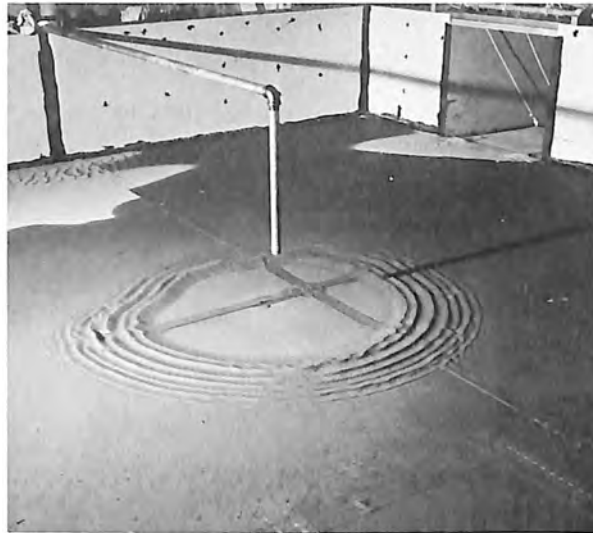
Figure 1. Test 1. Pattern of deposit resulting from initial operation of the slurry mixing and pumping system. Photo P801-D-73839
