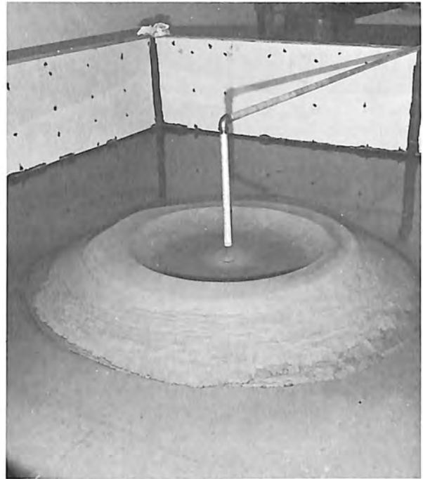
Figure 4. Test 4. Deposit pattern showing shear surface at the top of deposited cone. Water surface was held at the downslope elevation of the shear plane surface. Photo P801-D-73842
