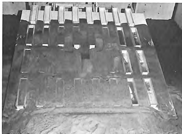
Figure 22. Test 12. Distribution of material on a 15^\circ slope with the water surface in the cavity higher than the injection pipe exit. Photo P801-D-73856
