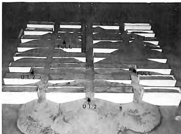
Figure 10. Test 8. Deposition pattern for corridors partially blocked and fully blocked at points indicated. Slurry concentration was about 35 percent, by weight. Corridor block designations are: U 1/2 indicates upper one-half of corridor is blocked; L 1/2 indicates lower one-half of corridor is blocked; full indicates full corridor is blocked. P801-D-73847
