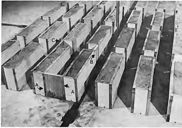
Figure 14. Test 10. Arrangement of pillars for backfill material pumped into a dry cavity. Blocks in one corridor were placed at A, B, and C as shown. Photo P801-D-73849
