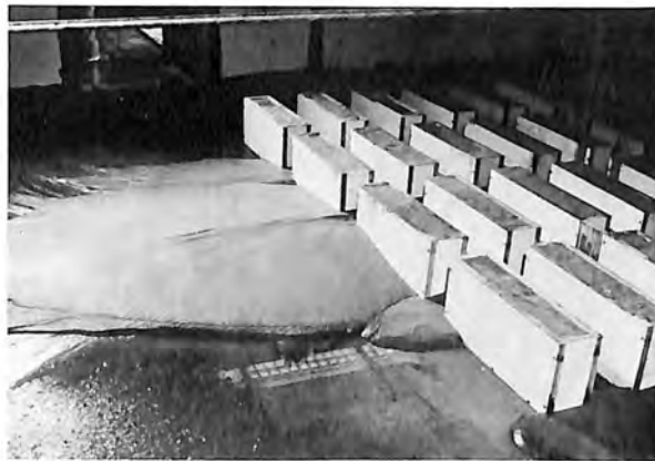
Figure 16. Test 10. Deposit at edge of pillar area shows slope of deposited backfill material for a dry cavity. Photo P801-D-73852
