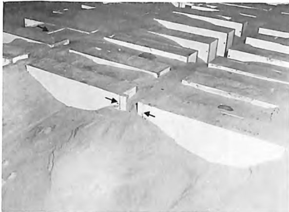
Figure 12. Test 9. Blocks to reduce flow areas by one-half in the corridors were placed at several locations (see arrows). Slurry concentration was approximately 25 percent with velocity in the injection pipe approximately 14 feet per second. Photo P801-D-73848
