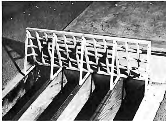
Figure 13. Lattice wall vortex suppressor. Photo PX-D-70837
