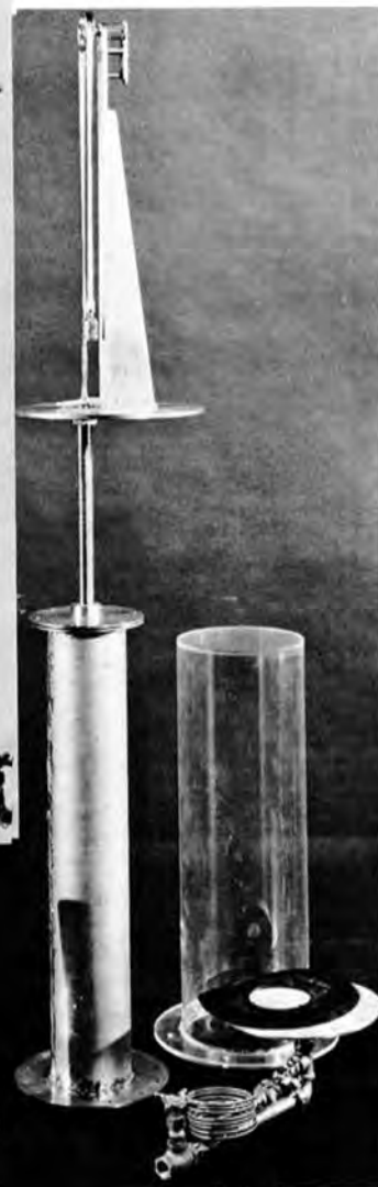
c. Stilling well parts except 2-1/2-inch float in well. Photo PX-D-70731
