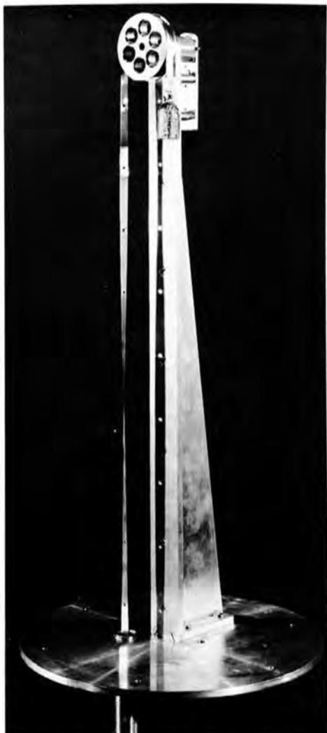
a. Float pulley on shaft of potentiometer, and perforated tape attached to float. Photo PX-D-70732
