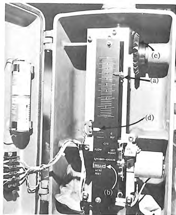
Figure 3. Vertical following pointer of newer-version device. Set point indicator (a). Totalizer dials (b). Set point hand crank and gear drive (c). Discharge indicator (d). Photo PX-D-70501
