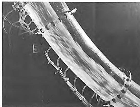
Figure 14. Recommended aeration slot, Station 7+79. Discharge is 50,000 cfs. The upper portion of the jet has spread to the tunnel walls and suppressed the side fins. Photo P459-D-68810
