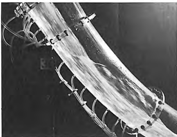
Figure 13. Recommended aeration slot, Station 7+79. Discharge is 30,000 cfs. These maximum side fins, one each side of the jet, do not reach the crown of the tunnel. Photo P459-D-68809
