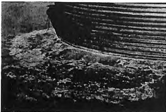
Photograph 13. Saturation condition around test tank containing natural, untreated soil. Such a condition will reduce seepage. Photo P800-D-68979
