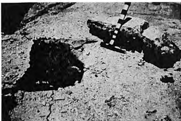
(a) Sample No. 1. Typical of best soil-cement. Photo P800-D-68968
