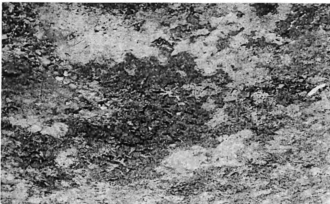
Photograph 10. Appearance of soil surface after ponding treatment with sealant B-6166. The material was applied at a rate of 2,000 pounds per acre (2,200 kg/ha). View shows that a major portion of the sealant did not penetrate the soil. Top photo P800-D-68973. Bottom photo P800-D-68974
