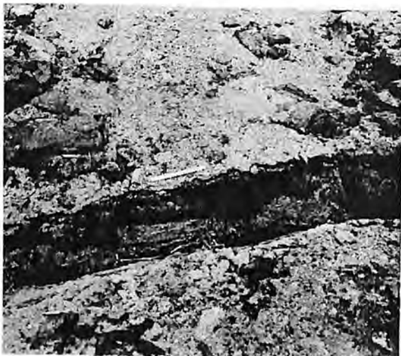
(b) Close-up view of asphalt penetration into natural soil. The 3-inch (7.6-cm) ruler is shown for comparison. Photo P800-D-68972
