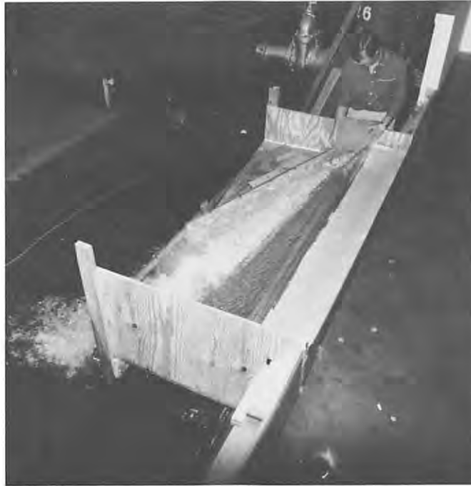
Figure 5c. - The 117° angled wall, ending 60 ft downstream from the dam at El. 6390.0—flow rate = 50% of the PMF.
