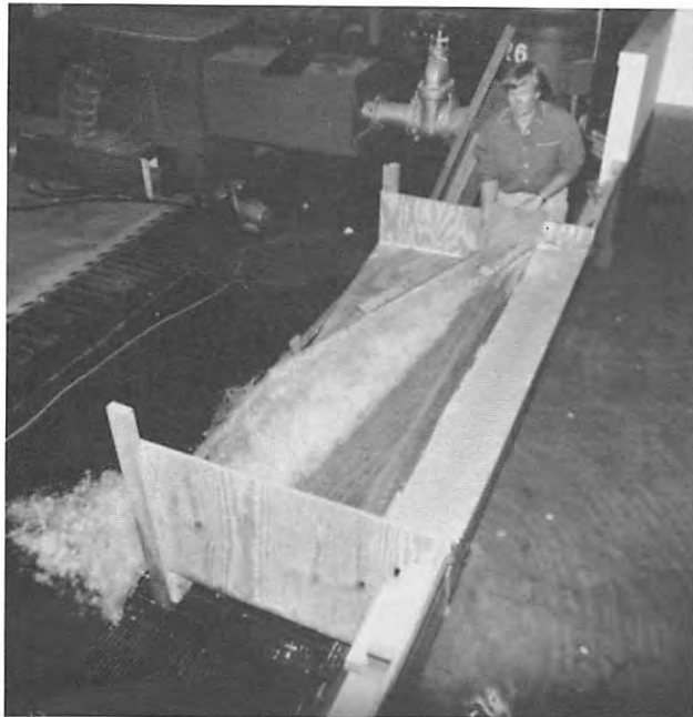
Figure 5a. - The 117° angled wall, with fillet, ending 60 ft downstream from the dam at El. 6390.0, showing the PMF flow rate contained by a 20-ft-high wall.
