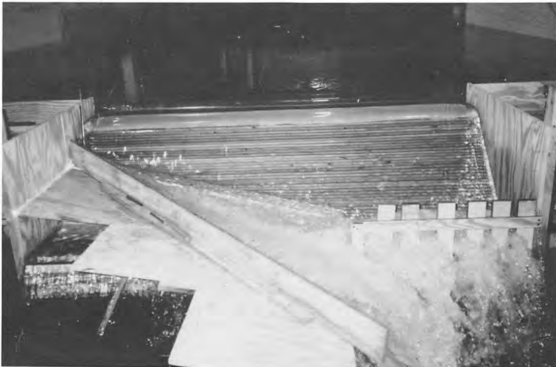
Figure 2. - The 1:36 scale right abutment model with the maximum wall angle tested.
