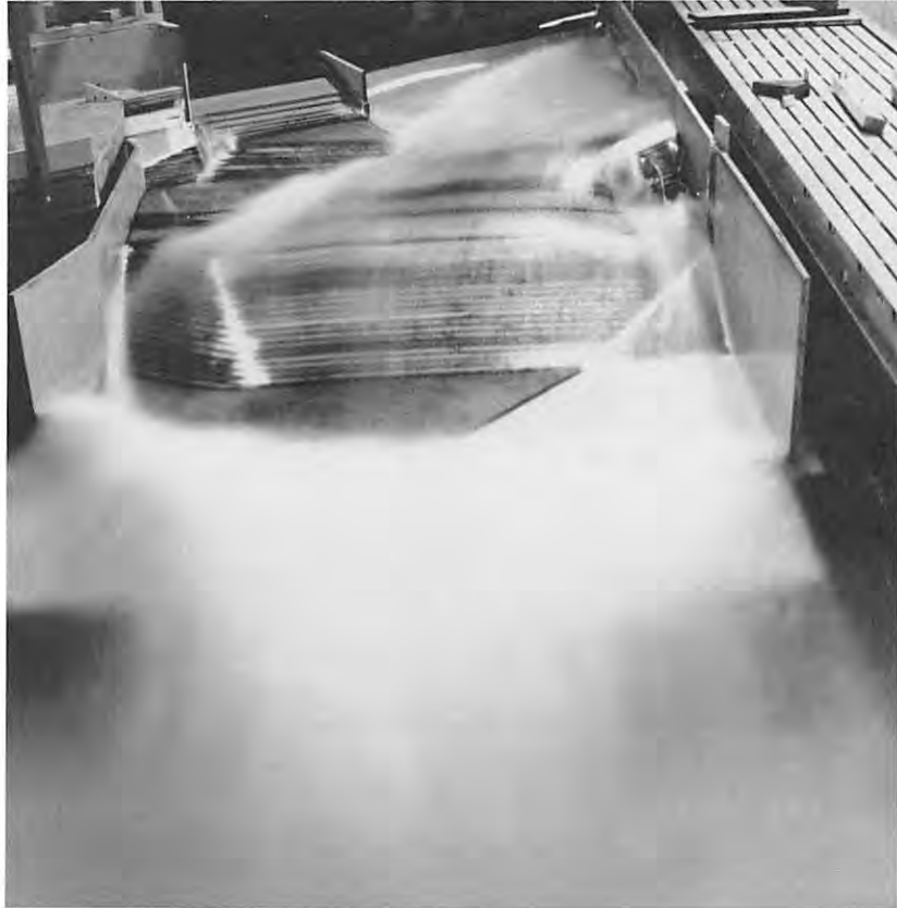
Figure 19b. - The recommended designs for the existing spillway at Black Rock dam operating under the PMF.
