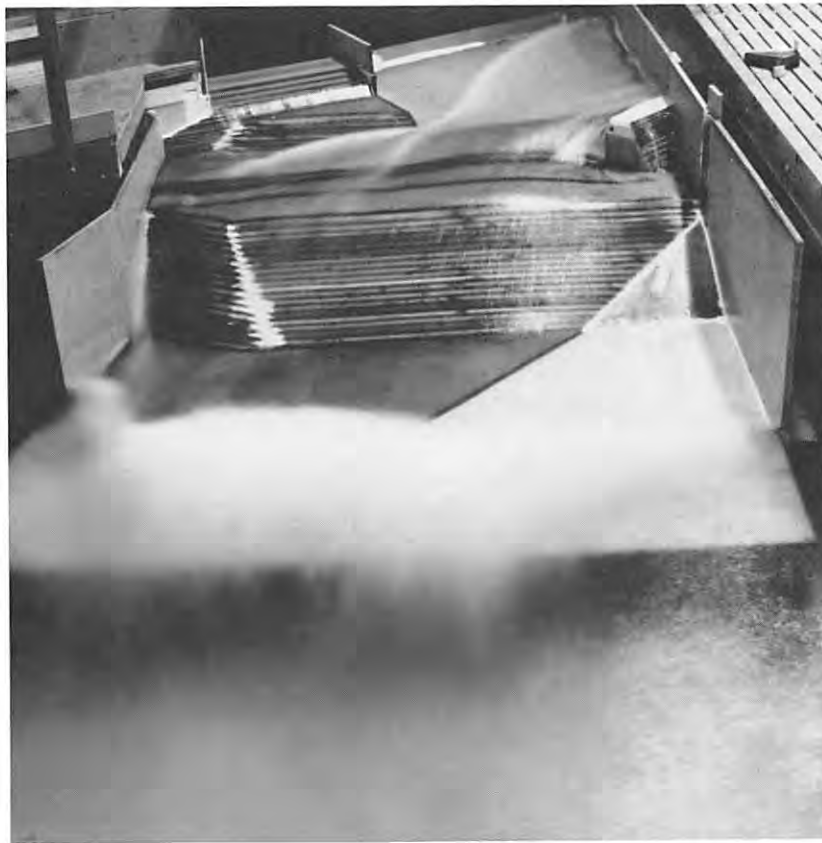
Figure 19a. - The recommended design for the existing spillway area operating under 50% of the PMF.
