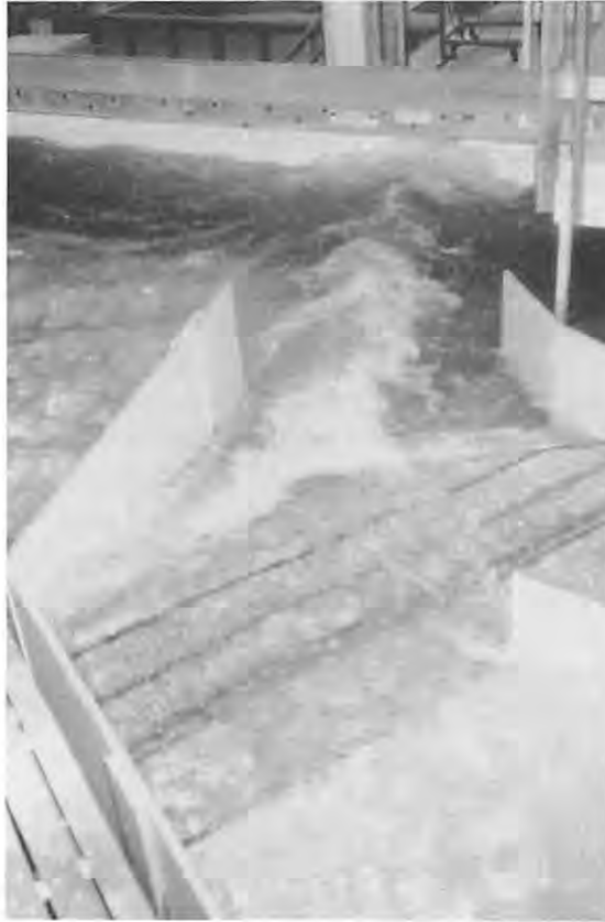
Figure 14. - PMF flow conditions downstream from the existing spillway with the wall angled across the apron toward the river channel.
