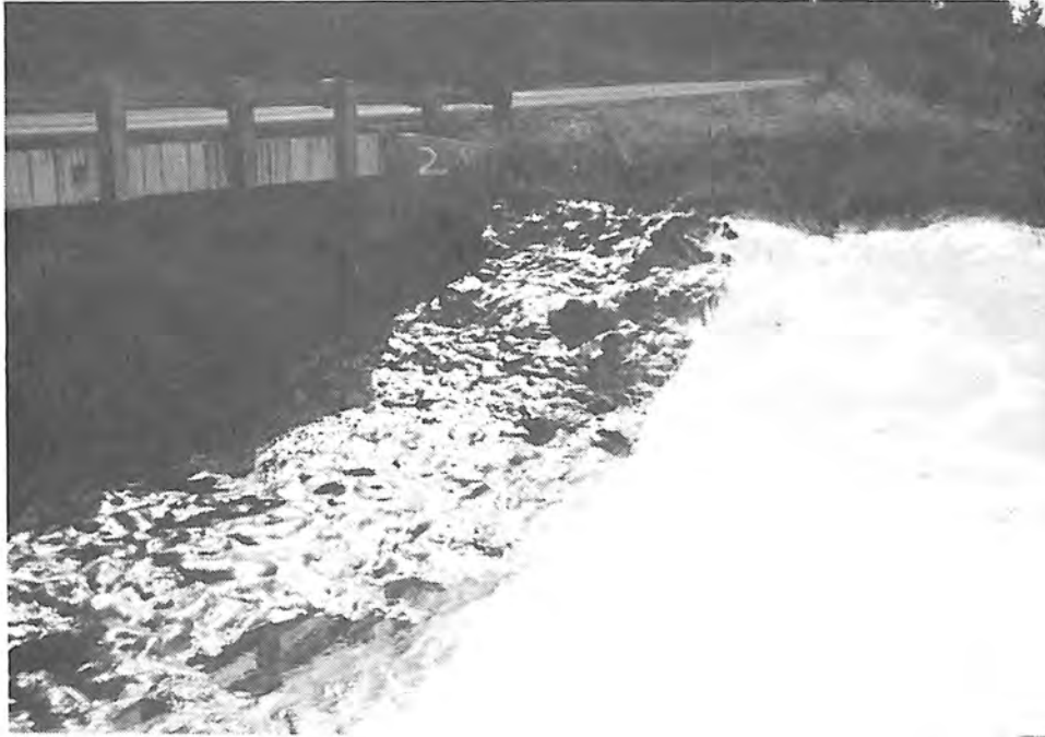
Photograph 71. — Black Geothane 5020 applied at left; white Futura 500/550 applied at right.
