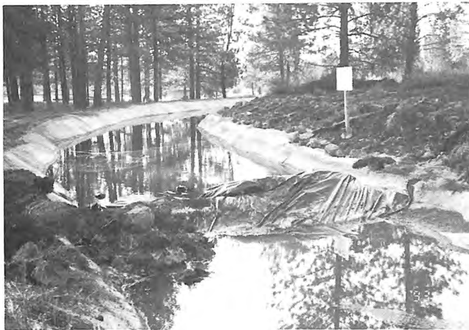
Photograph 111. — Typical dike construction for ponding tests over installed materials.
