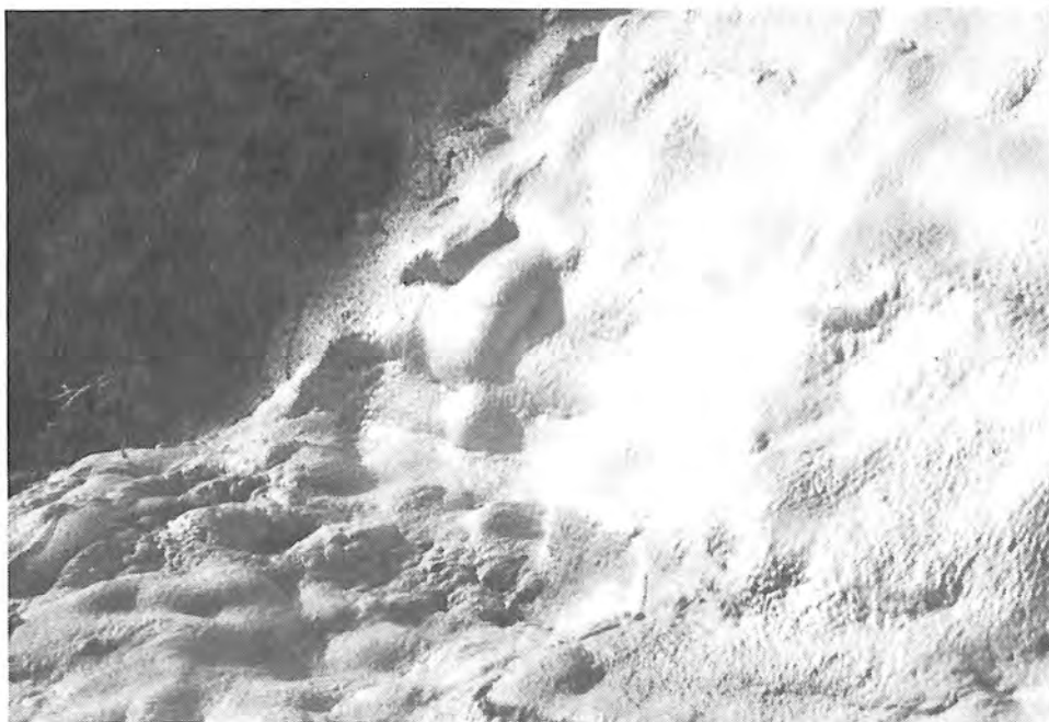
Photograph 68. — Dark area on left is 2-pound foam beneath newly applied 5-pound foam, on right.
