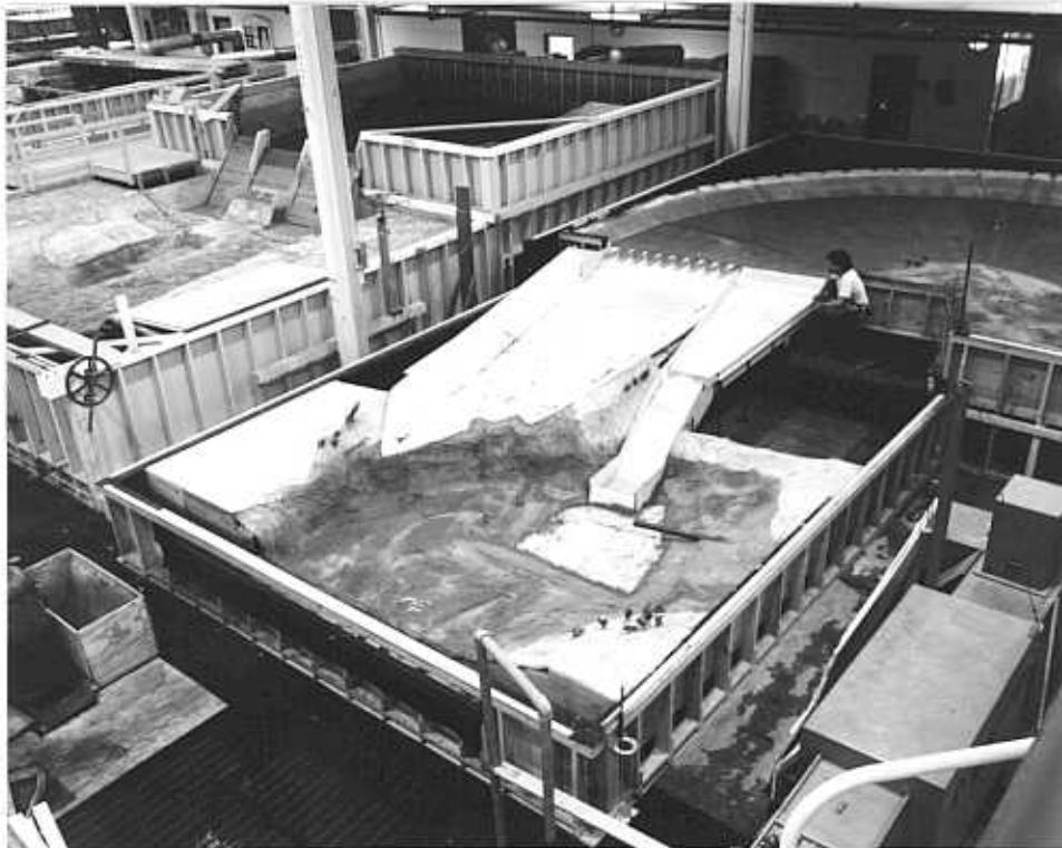
Figure 2. - Ritschard Dam hydraulic model.
