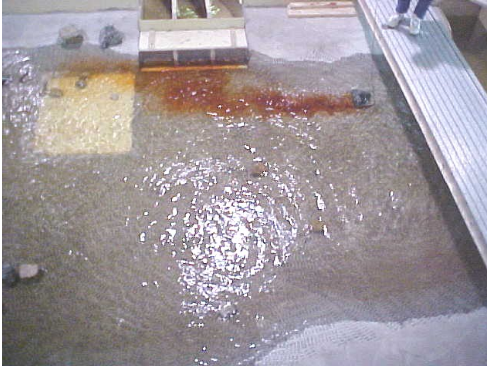
Figure 16. Dye injection upstream of DPP intake
