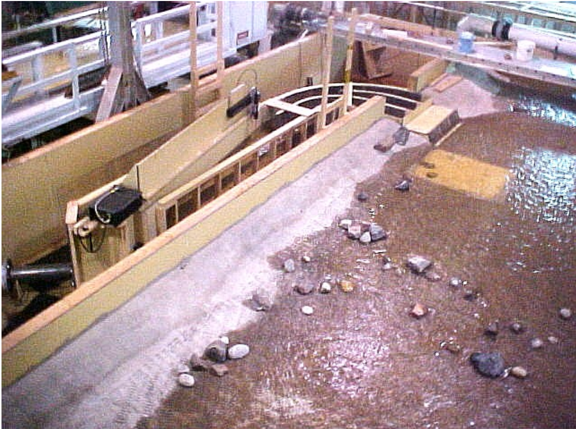
Figure 4. 1:12 scale model of the Durango Pumping Plant intake structure
