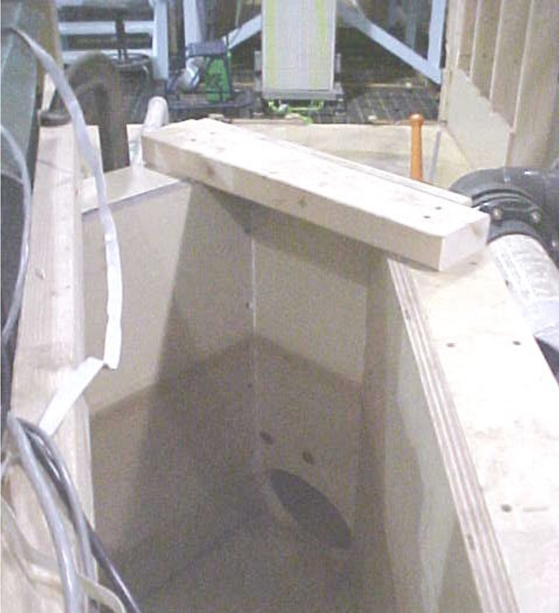
Figure 14. Pump intake forebay during model operation Flow conditions in photo: Stream Q = 580 \text{ ft}^3/\text{s} Pump Q = 280 \text{ ft}^3/\text{s}
