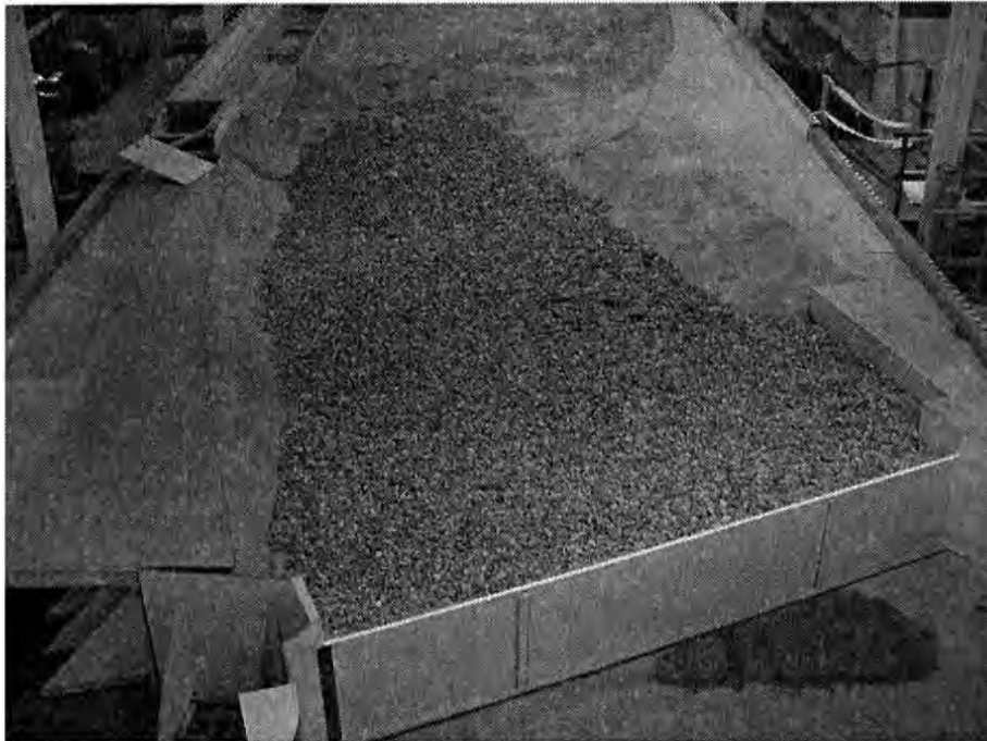
Figure 3. - Photograph of PSDD physical model as constructed at Reclamation's Water Resources Research Laboratory in Denver, Colorado.
