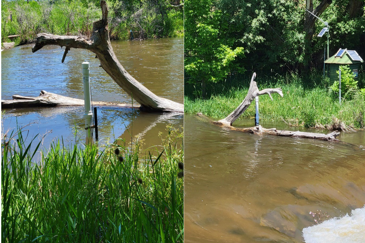
Figure 10 – Photographs showing the eTape® sensor installed at the Boulder Creek location.
