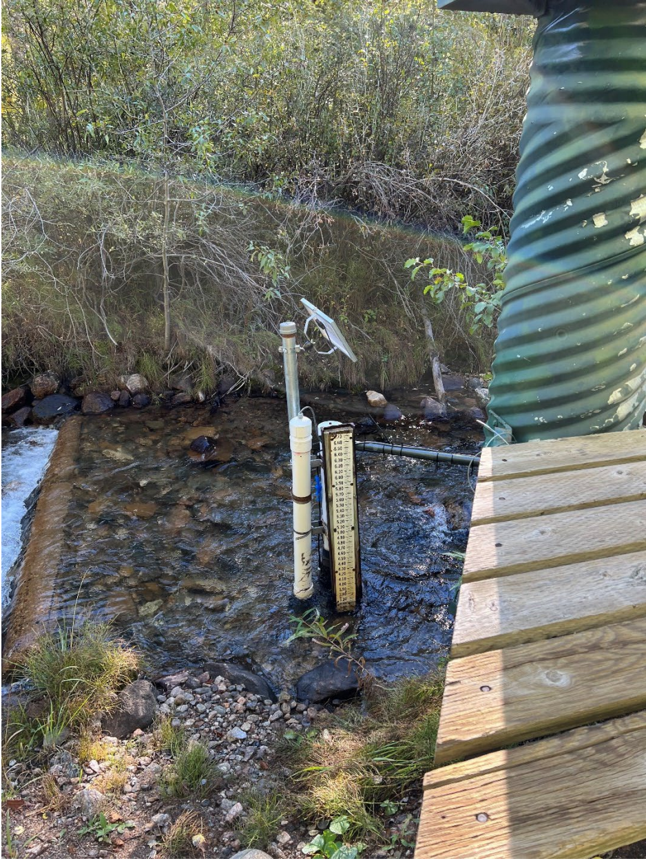
Figure 12 – Photograph showing the eTape® sensor installed at the Leavenworth Creek location.
