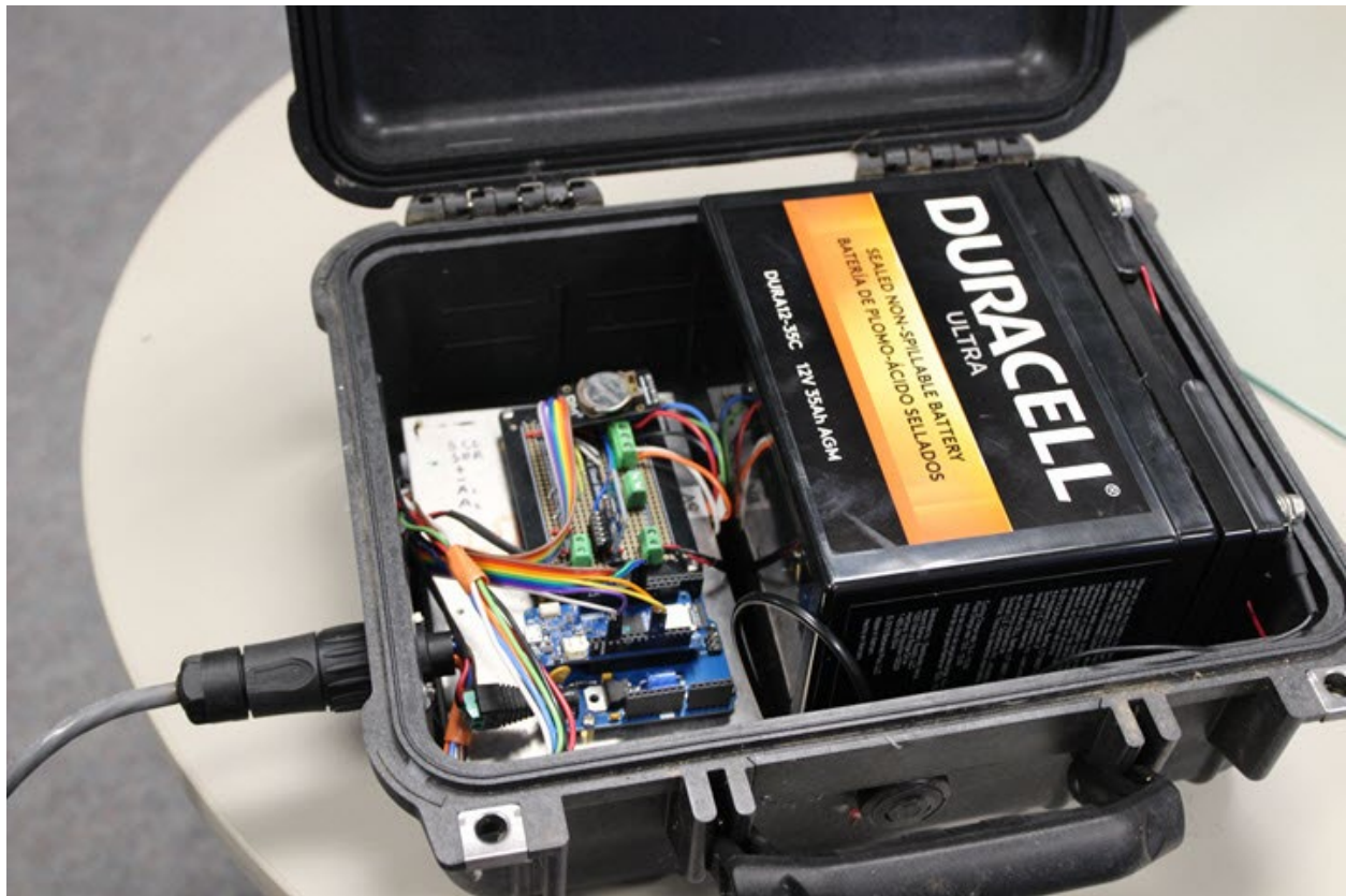
Figure 8 – Photograph of the entire datalogger assembly showing the backplane assembly along with a 12 VDC, 35 amp-hr battery. A water-tight connector (left) was used for connecting the eTape®.
