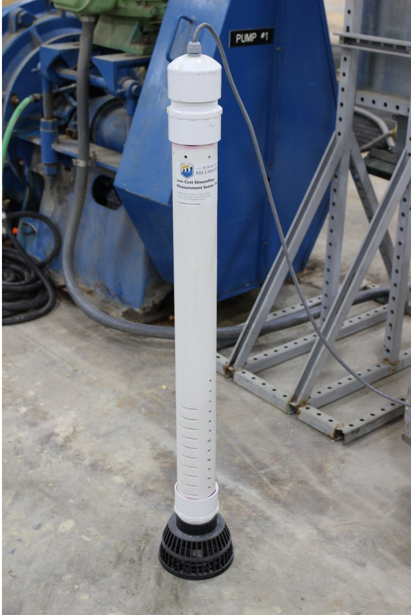
Figure 2 – Photograph of the PVC standpipe housing the eTape®.
