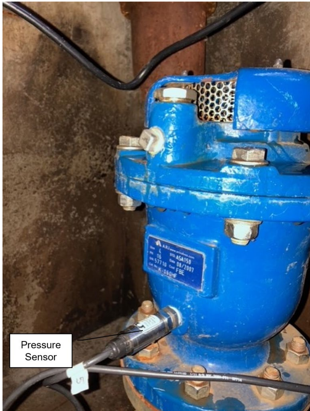
Figure 2 Pressure sensor mounted on the downstream side of the 4-inch air valve to measure pipe pressures directly downstream of the slide gate.
