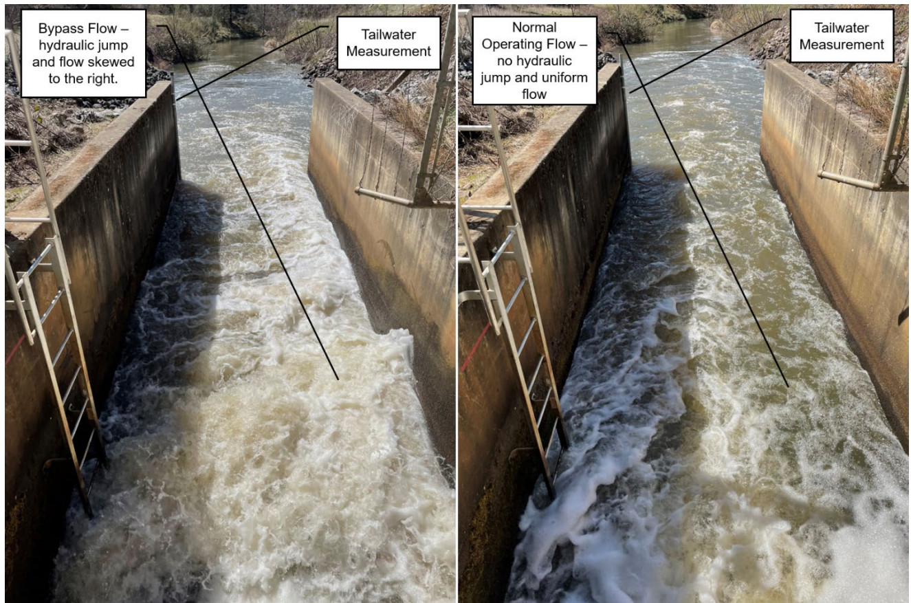
Figure 14 Flow conditions in the powerplant tailrace (looking downstream) for approximately 70 cfs in both bypass mode (left) and normal power generation mode, post-test (right).
