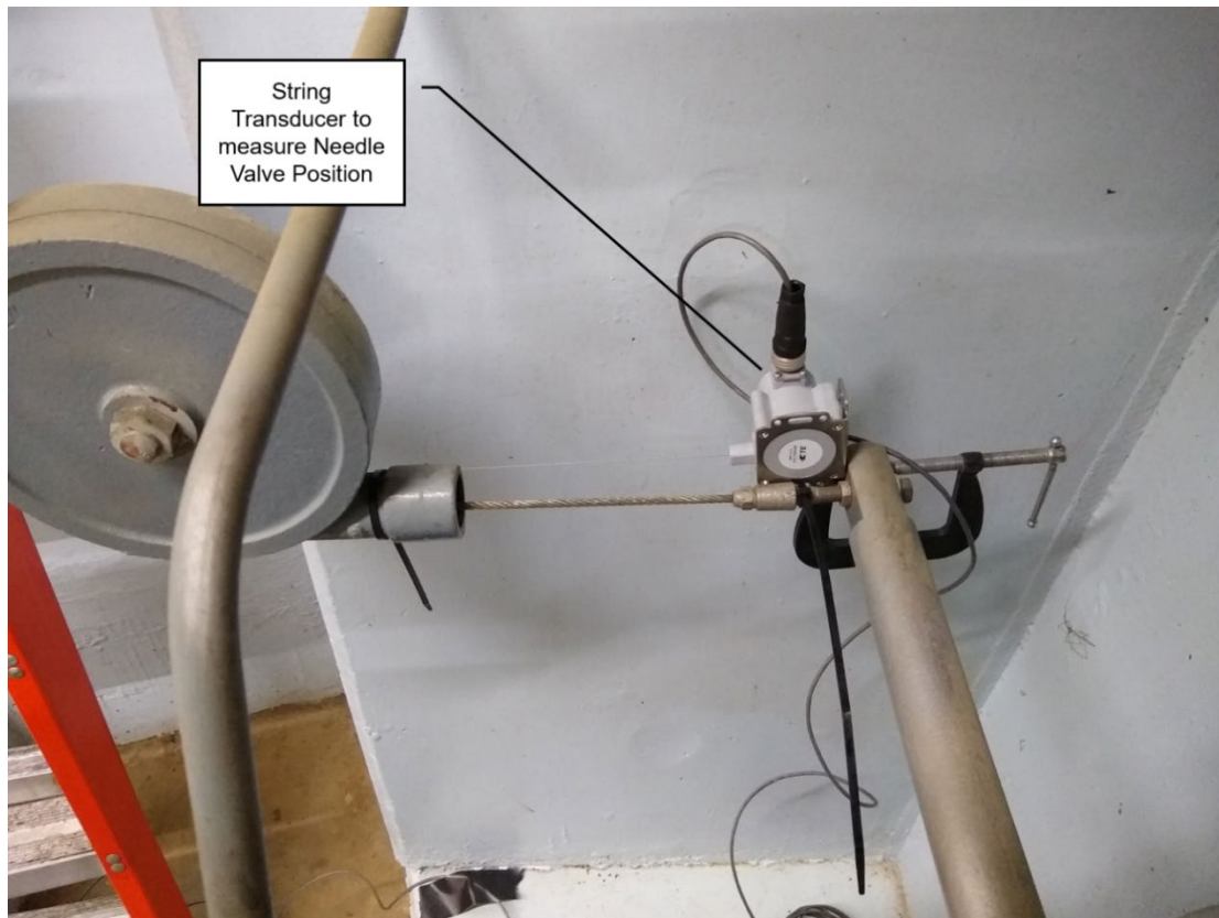
Figure 5 String transducer used to measure the position of the Turbine Needle Valve 4.
