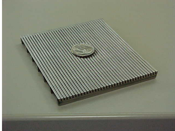
Figure 2. — Sample section of a Coanda-effect screen panel. The slot size is 0.5 mm.
