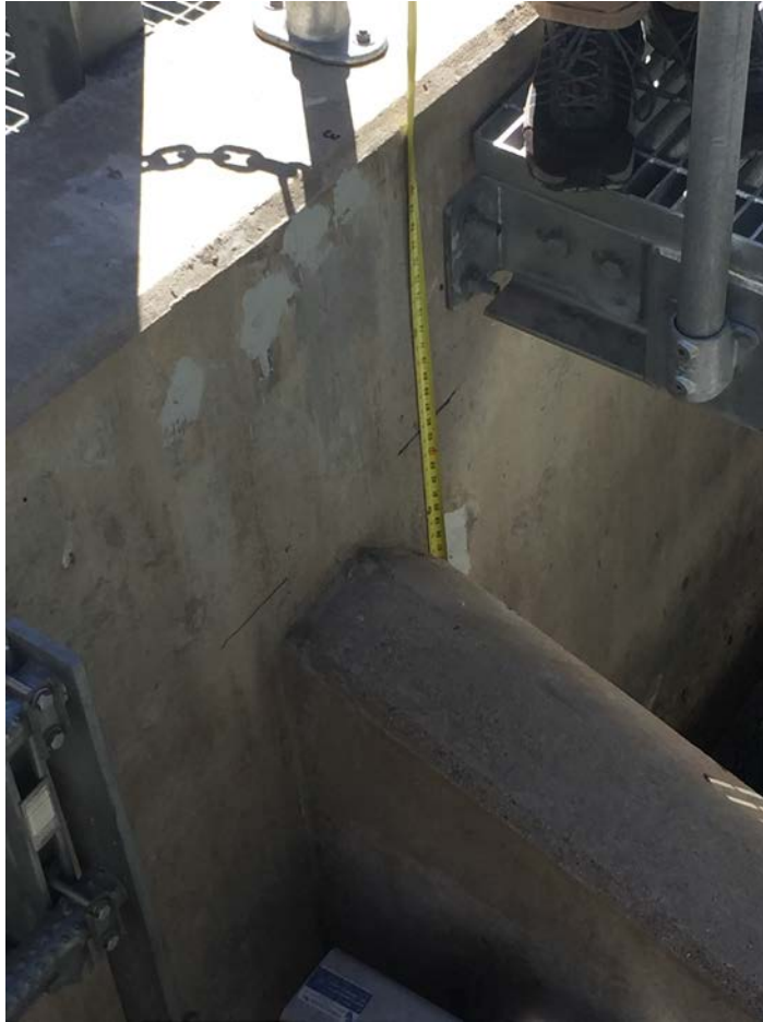
Figure 19. Photograph of fish ladder pool differential measurements by level line and tape measure
