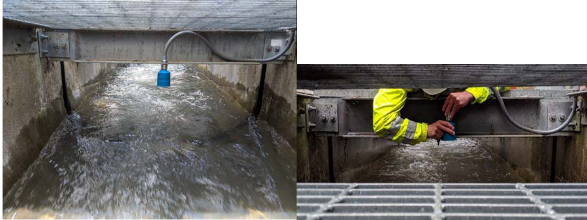
Figure 20. Photographs of SS5 showing original sensor mount (left image) and temporary relocation (right image) to test sensor deadband errors
