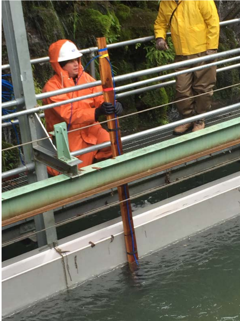
Figure 4. Photograph of ADV data being collected at ECDD showing the red tape mark on the 2x4 that was used to ensure correct measurement depth.
