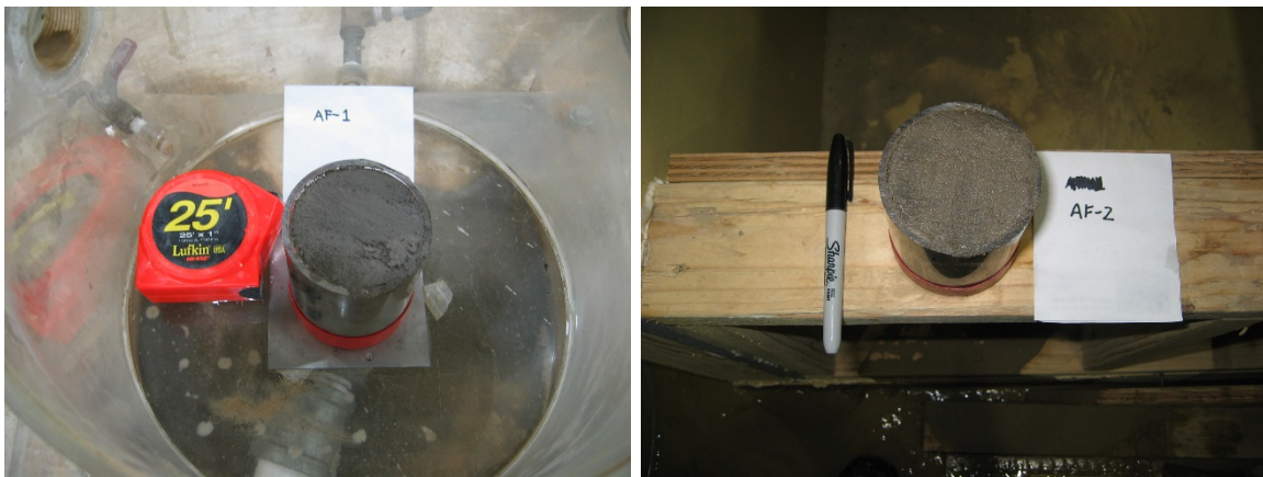
Figure 2. — Representative jet test specimens from American Falls Reservoir, prior to testing.
