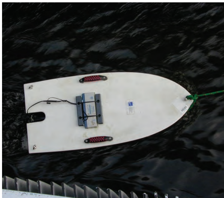
FIGURE 8.—Nortek BoogieDopp velocity profiler.
