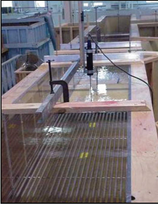
FIGURE 2.—Passive separator model bar rack at a 0° angle leading into raceway.
