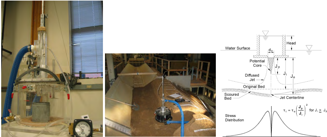
Figure 1. — Submerged jet erosion test device for laboratory and in situ use, and a schematic diagram including the stress profile applied to the soil boundary (Hanson and Cook 2004).
