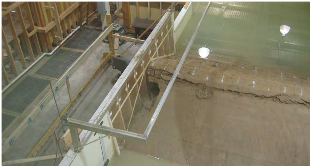
Figure 8. Post-test overhead view of the entrance to the internal erosion flow channel.
