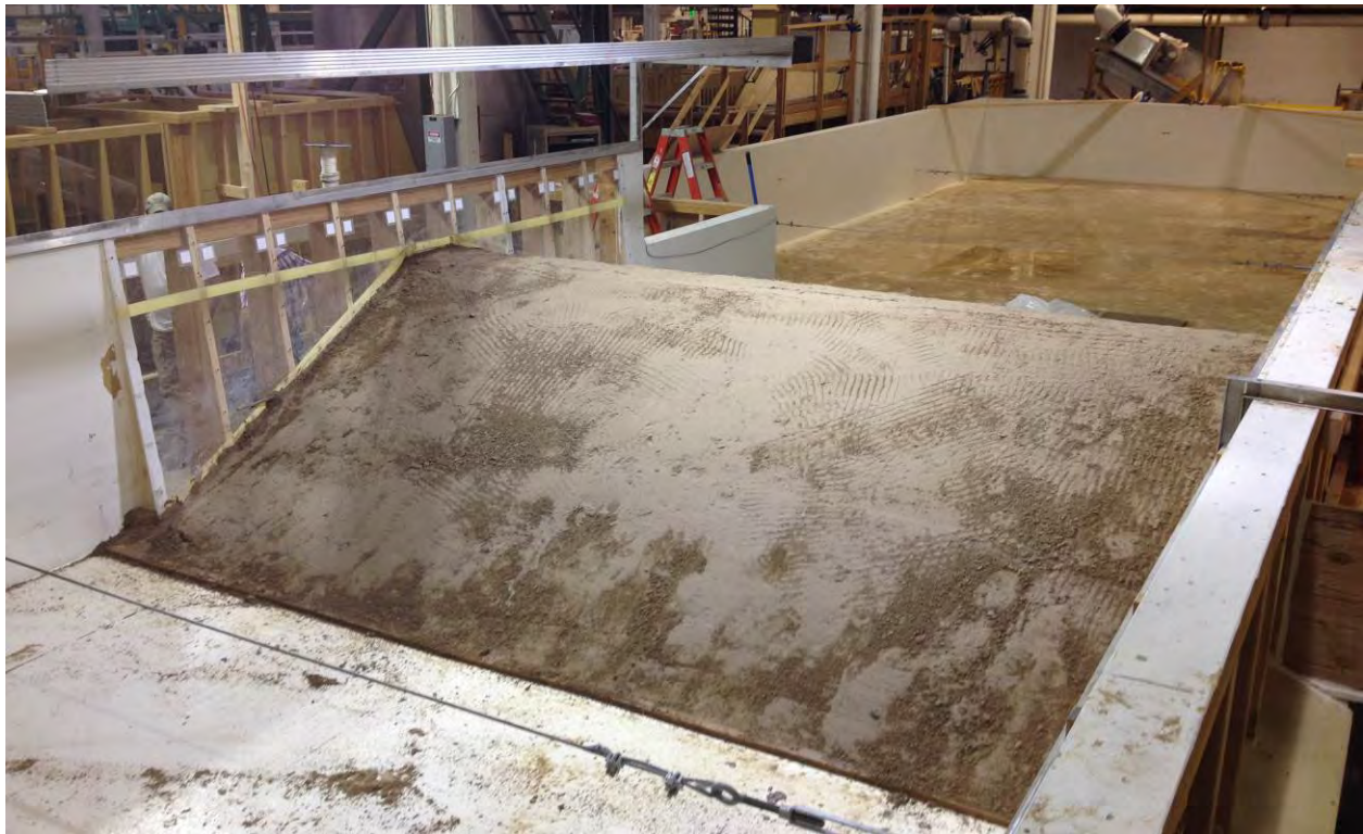
Figure 1. Embankment breach test facility viewed from the upstream end of the headbox, overlooking the completed test embankment.
