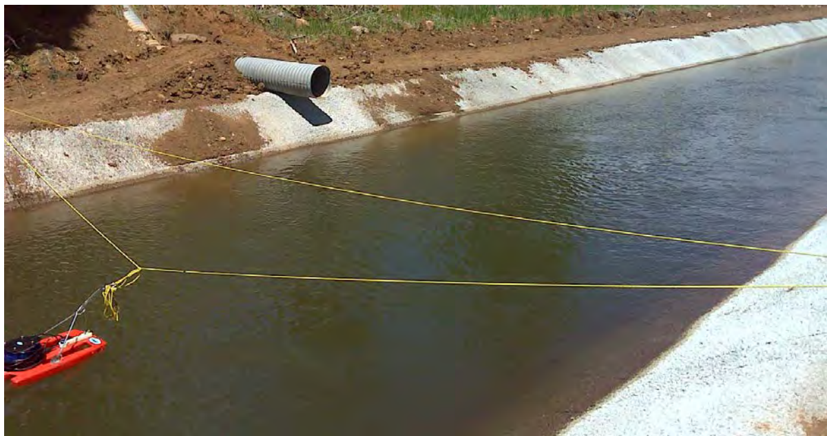
Figure 8. Photograph of the flow measurement cross section upstream from the Payne Canyon Siphon (flow is from right to left). The Teledyne/RDI Streampro and tagline were installed at the same location as pre-project measurements.
