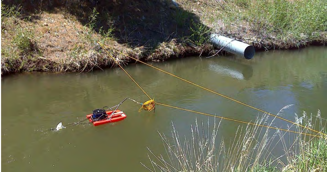
Figure 2. Photograph of the flow measurement cross section upstream from the Payne Canyon Siphon (flow is from right to left). The Teledyne/RDI Streampro and tagline were temporarily installed for this flow measurement.
