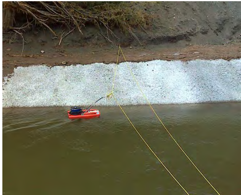
Figure 9. Photograph of Streampro measurement located 640 ft downstream from the start of canal lining. This location was selected to be an adequate distance downstream from a bend in the canal, N37°17'24.4" W107°47'46.5".
