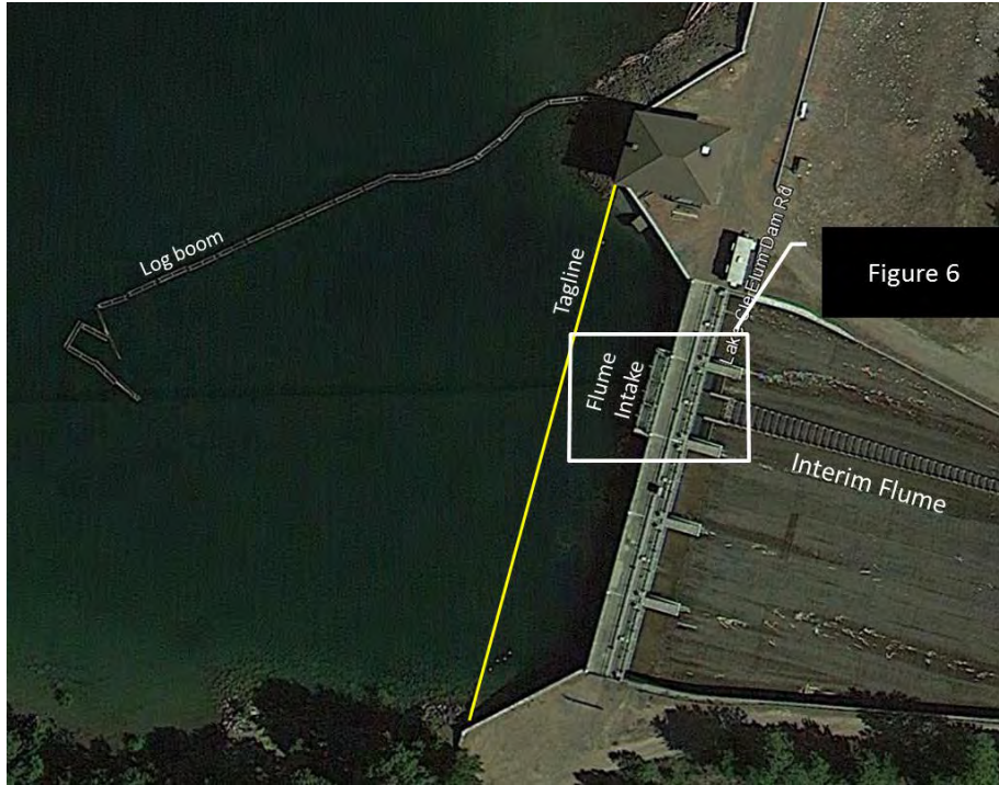
Figure 5. Aerial photograph of the Cle Elum interim flume intake and tagline location. During the measurements the log boom was spanning the approach channel. The box indicates the extents of figure 6. (Image date: November 6, 2012).
