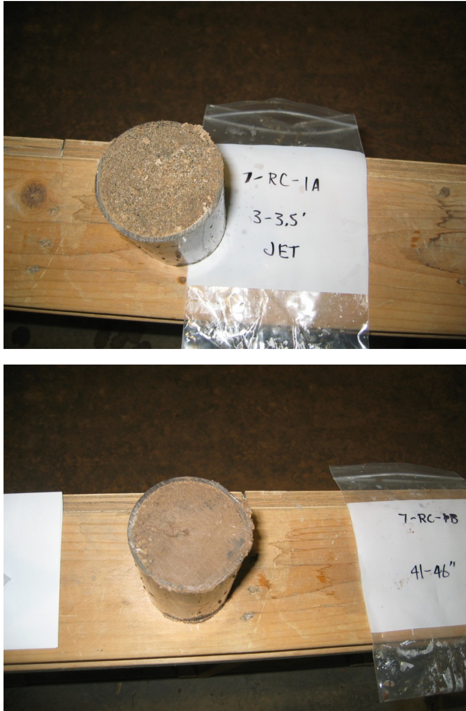
Figure 2. — Representative jet test specimens from Paonia Reservoir, prior to testing. Specimens like the sandy soil at top were usually completely eroded to the bottom of the tube in less than 1 to 2 minutes.
