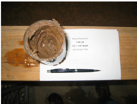
Figure 3. — Post-test photographs of jet test specimens that exhibited some erosion resistance. Most of these specimens were tested for about 30 – 60 minutes.
