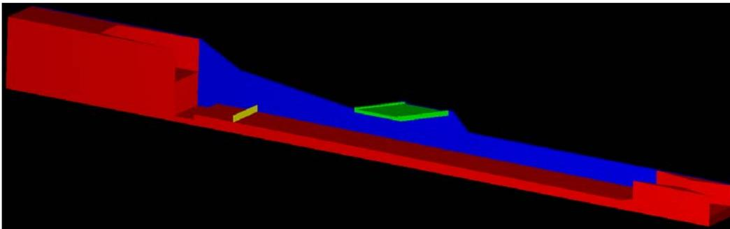
Figure 10. — 3-ft-high stoplog baffle located 30 ft downstream from vertical drop. The near wall of the approach channel is not shown.
