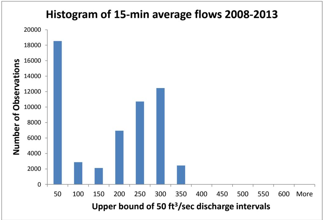
Figure 4. — Frequency histogram of the flows from the Homestake Tunnel over the past 6 years. Bars show the number of flows observed in intervals of 1-50 ft<sup>3</sup>/sec, 51-100 ft<sup>3</sup>/sec, etc. Conditions of exactly zero flow (approx. 153,000 observations) are not included.
