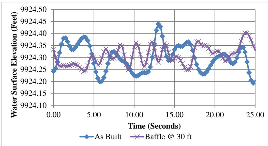
Figure 14. — Simulated waves upstream from Parshall flume, comparing baffle at 30 ft to as-built condition.
