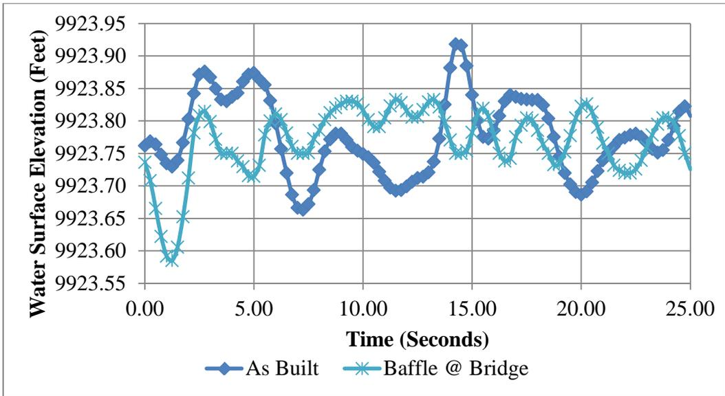
Figure 19. — Simulated waves at (2/3)A location in Parshall flume, comparing baffle at bridge to as-built condition.
