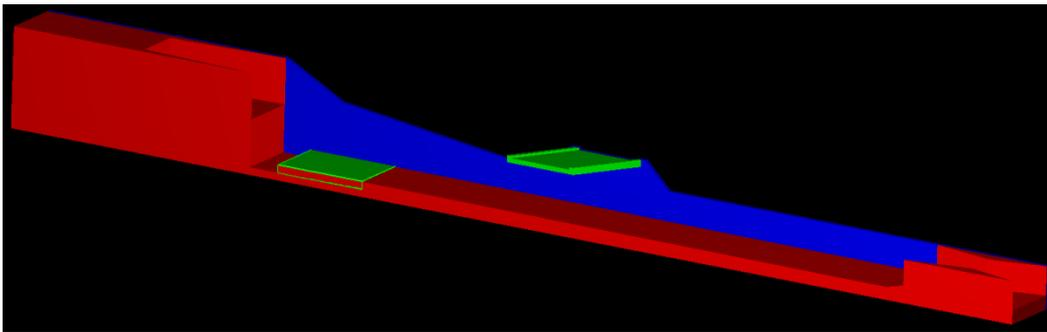
Figure 8. — Modified stilling basin configuration (green box highlights existing concrete that would be removed). The near wall of the channel is not shown.
