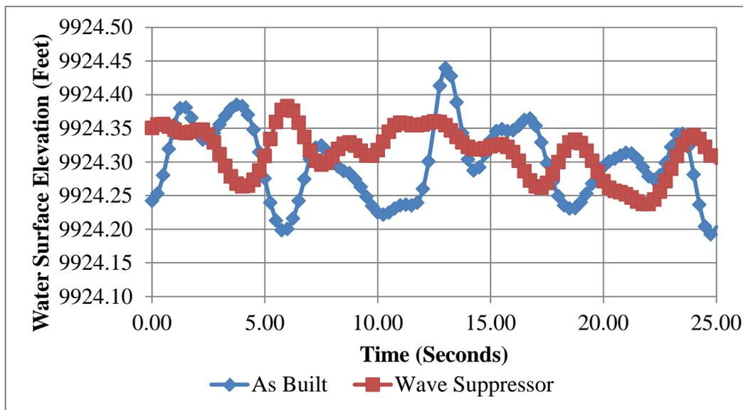
Figure 12. — Simulated waves upstream from Parshall flume, comparing wave suppressor to as-built condition.
