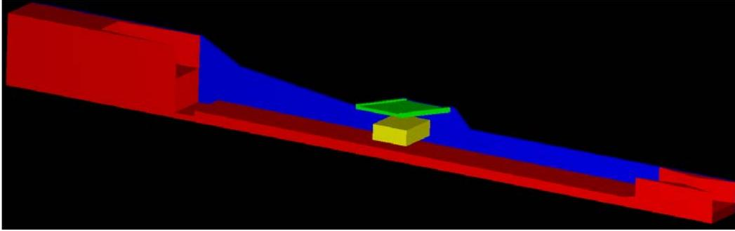
Figure 6. — Wave suppressor configuration. Near wall of approach channel is not shown.
