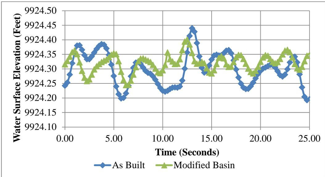
Figure 13. — Simulated waves upstream from Parshall flume, comparing modified stilling basing to as-built condition.
