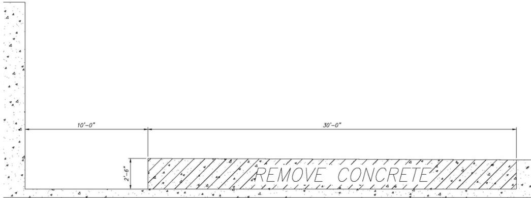
Figure 9. — Modified stilling basin dimensions.
