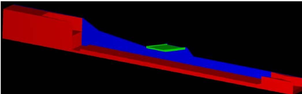
Figure 5. — As-built configuration. The near wall of the flume approach channel is not shown in order to make approach channel details visible.
