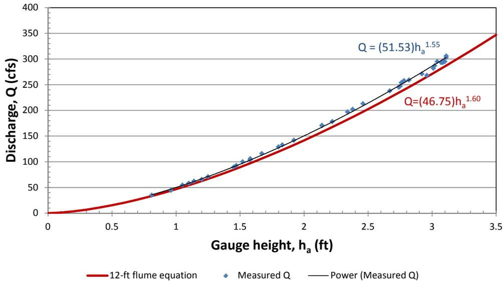
Figure 2. — Discharge measurements since 1999 compared to standard free-flow rating equation for a 12-ft Parshall flume.
