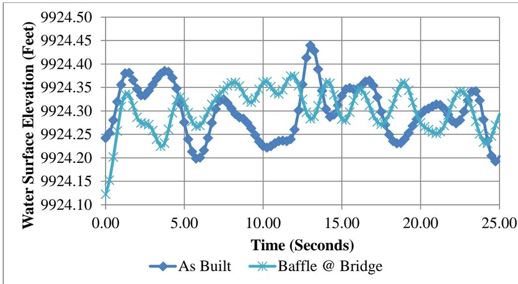
Figure 15. — Simulated waves upstream from Parshall flume, comparing baffle at bridge to as-built condition.
