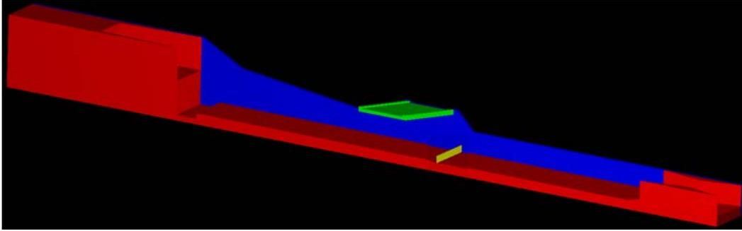
Figure 11. — Stoplog baffle located beneath road bridge, as tested in 2013. The near wall of the approach channel is not shown.
