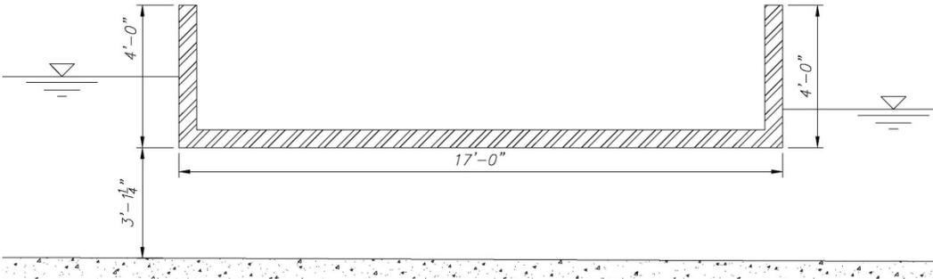
Figure 7. — Dimensions of an underpass wave suppressor designed for the Homestake channel with a discharge of  $300 \text{ ft}^3/\text{sec}$ .
