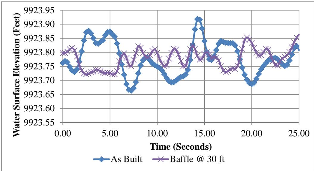
Figure 18. — Simulated waves at (2/3)A location in Parshall flume, comparing baffle at 30 ft to as-built condition.
