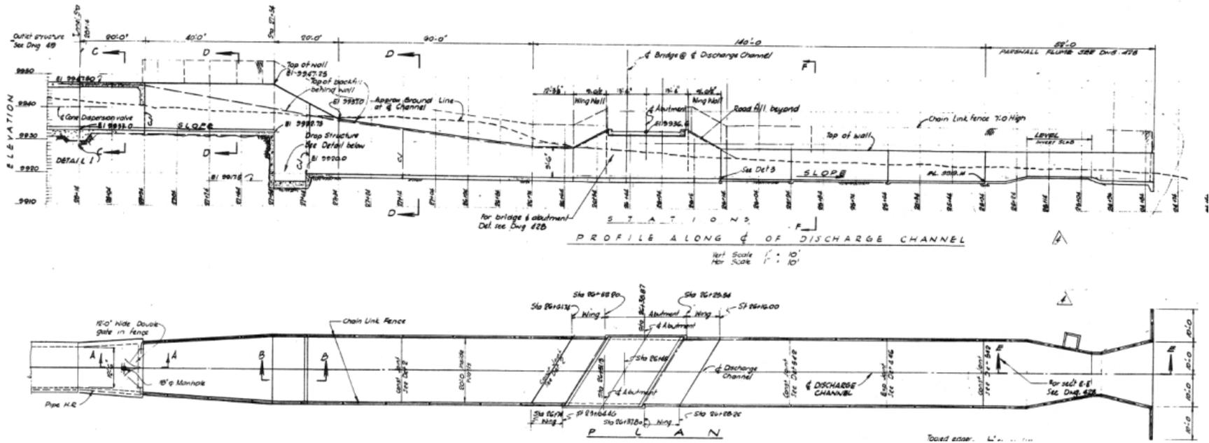
Figure 1. — Homestake Tunnel outlet structure and flow measuring flume. The Howell-Bunger valve is located just to the left of this drawing.
