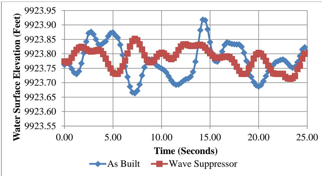
Figure 16. — Simulated waves at (2/3)A location in Parshall flume, comparing wave suppressor to as-built condition.
