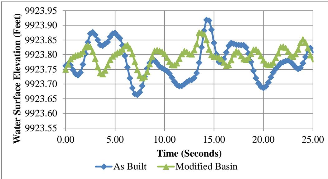
Figure 17. — Simulated waves at (2/3)A location in Parshall flume, comparing modified stilling basin to as-built condition.
