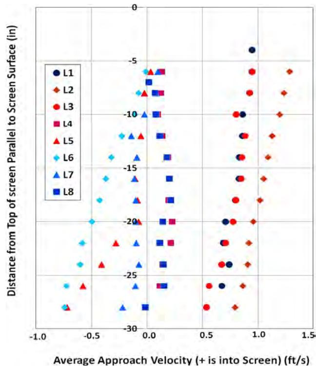
Figure 4. Baseline condition tested in 2010 [1] with no Baffle --- Cone Screen approach velocity profiles measured at locations L1 through L8.
