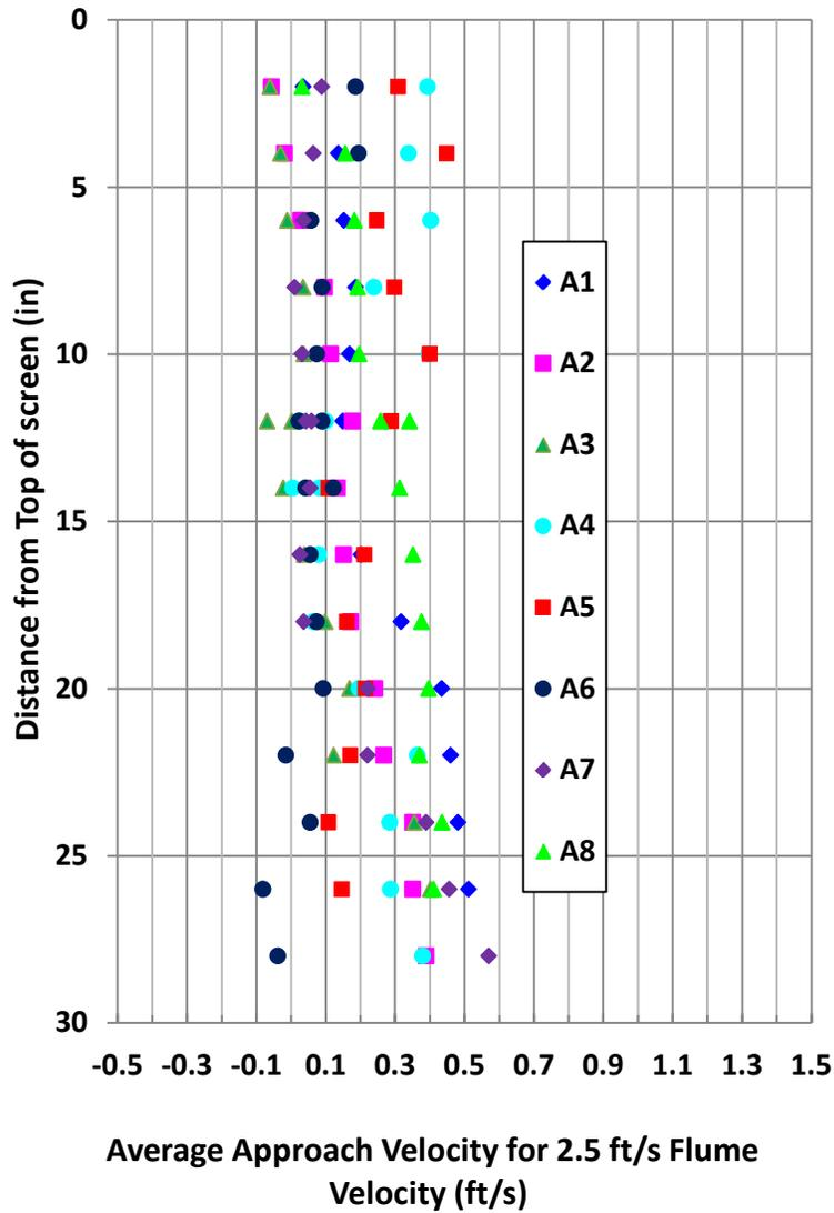
Figure 8. Bullnose Concept 1 - Cone screen approach velocity profiles measured at locations A1 through A8.
