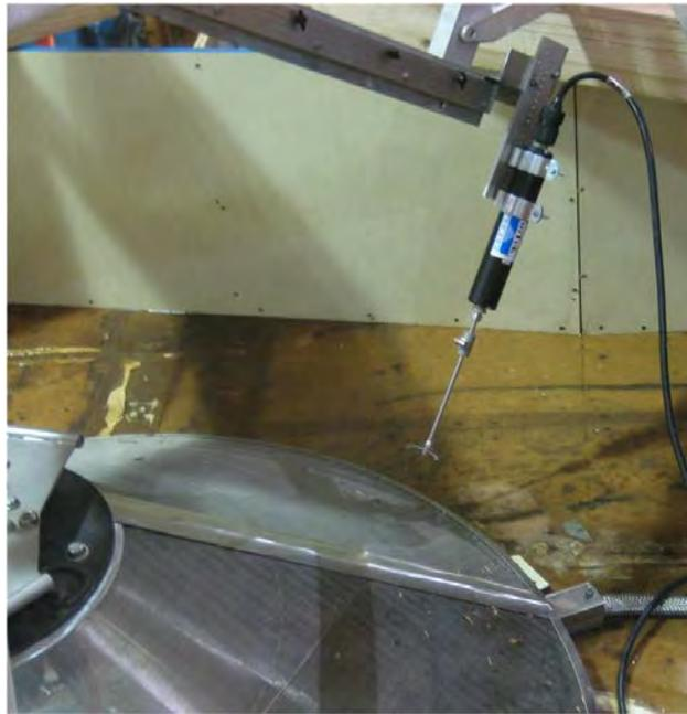
**Figure 2. Sontek ADV probe test apparatus**
