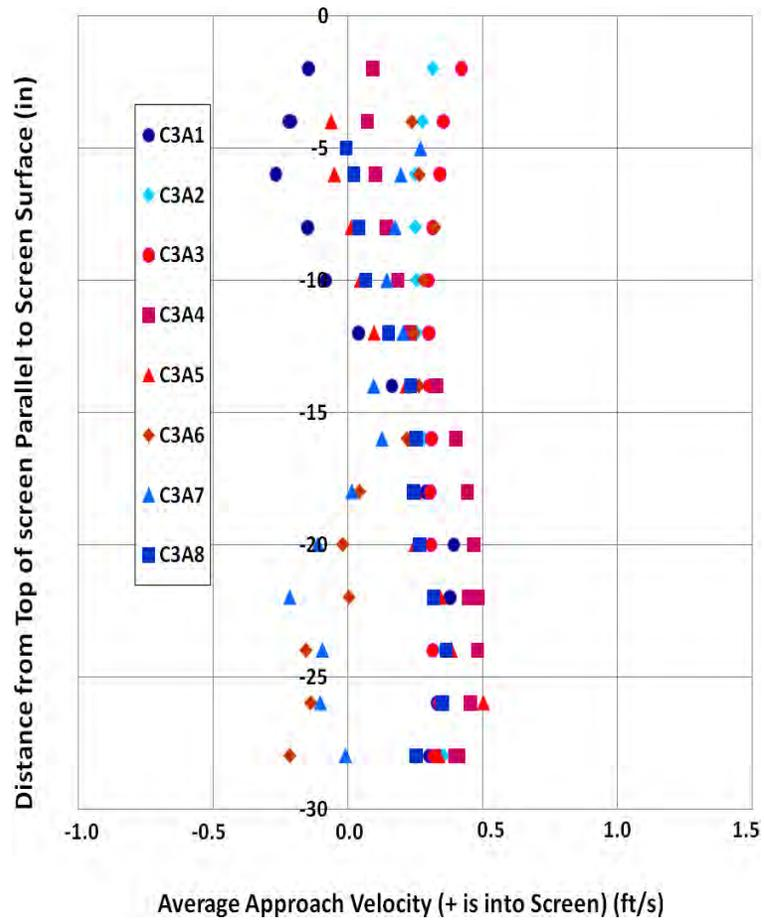
Figure 15 Internal Baffle Concept 3 with 2 ft/s flume velocity - Cone screen approach velocity profiles measured at locations A1 through A8.
