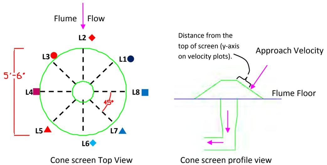
Figure 3. Velocity measurement locations for baseline condition and profile view of the screen setup.
