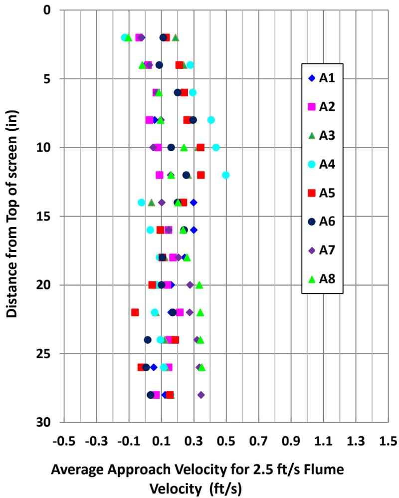
Figure 11. Bullnose Concept 2 - Cone Screen approach velocity profiles measured at locations A1 through A8.
