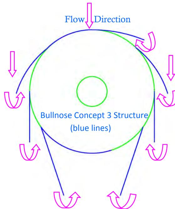
**Figure 12. Illustration of Bullnose Concept 3. Blue lines indicate bullnose structure.**
