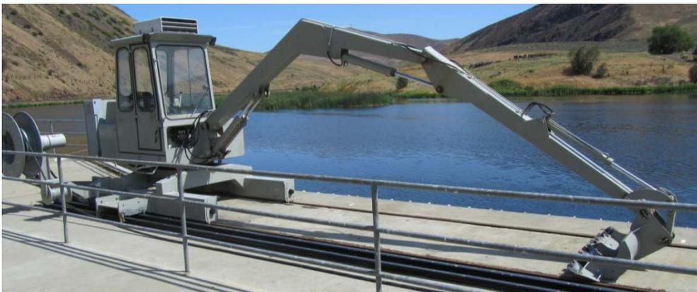
Figure 2 - Backhoe style rake on deck rails at the Roza Dam trashrack
