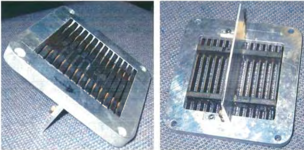
Figure 6. — Test screen B-1 in mounting block and a view of the underside of the screen with divider plate installed. Flow is left to right in both photos.
