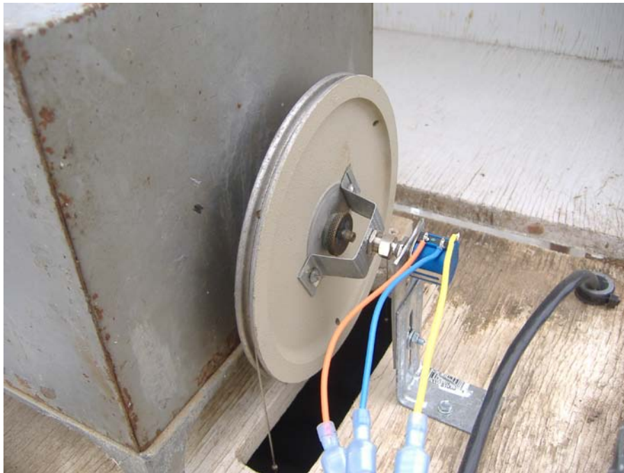
Figure 4. A Potentiometer Mounted to a Stevens type F Recorder Pulley
