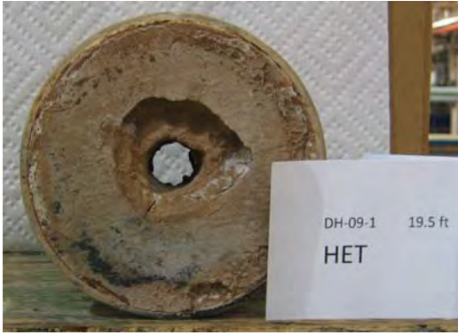
Figure 1. — Post-test photo of HET specimen from sample 37Q-160, DH-09-01, depth 19.5 ft.
