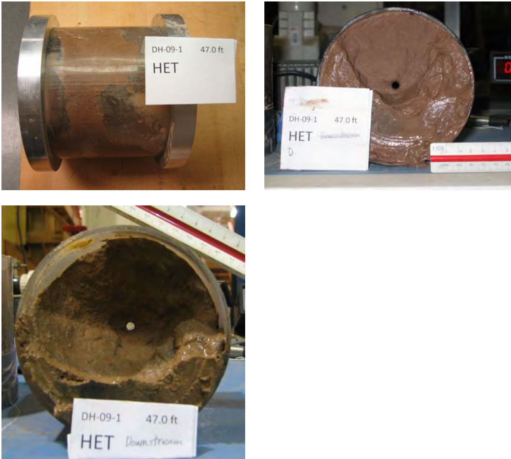
Figure 5. — Several views of HET specimen from sample tube 37Q-171, following erosion test. Clockwise from top-left: top view through specimen tube showing clay lens left of center (flow right to left); upstream end of specimen; and downstream end of specimen.
