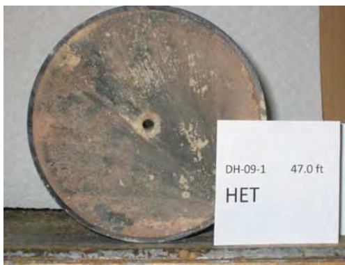
Figure 4. — Photograph of HET specimen from sample tube 37Q-171 prior to erosion test.
