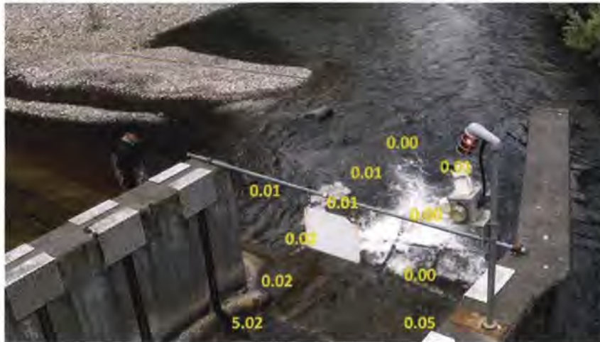
Figure 6. Voltage gradient measurements downstream of the low flow channel, between the main deck of the electrical barrier and the fish ladder.
