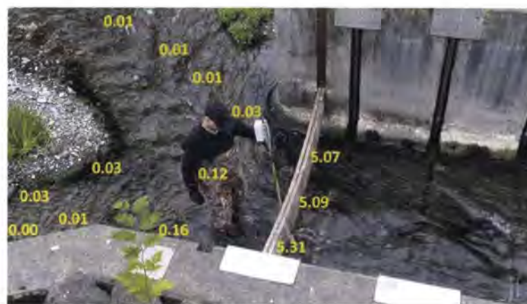
Figure 5. Voltage gradient measurements upstream of low flow channel and over the furthest most upstream anode located next to the main deck of the concrete slab electrical barrier.
