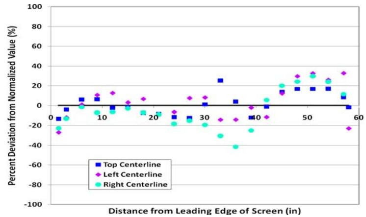
Figure 4. Percent deviation from normalized value for the right, left and top centerline approach velocities – WTEV75 configuration.
