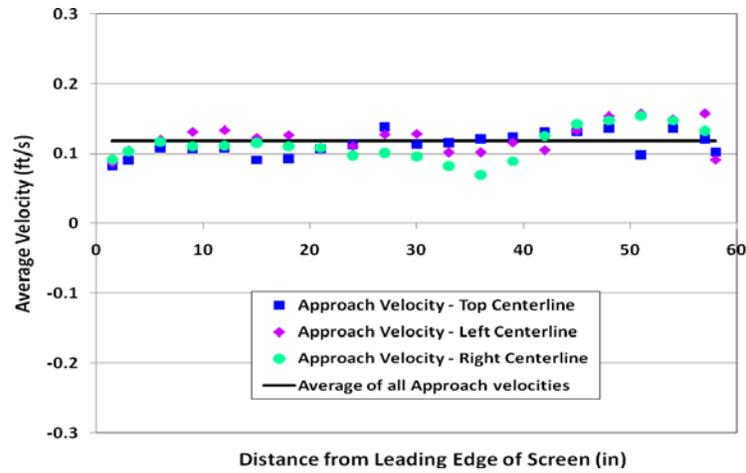
Figure 3. Approach velocities measured 3 in from the screen face, along the top, left and right centerlines for the WTEV75 configuration.
