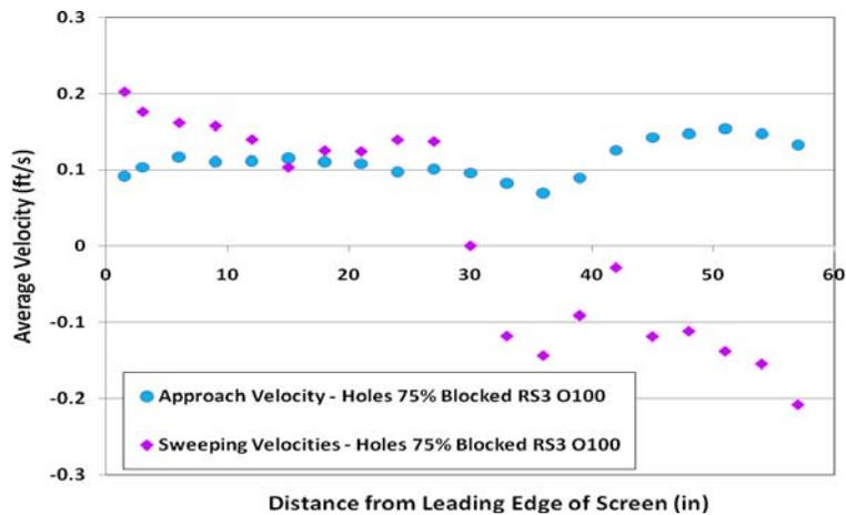
**Figure 6.** Approach and sweeping velocities measured 3 inches from the screen along the right side (RS3) centerline – WTEV75 configuration.
