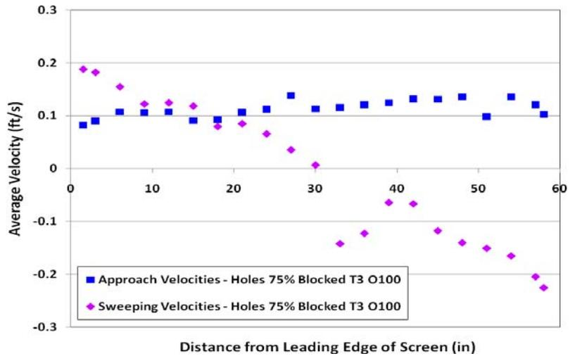
**Figure 7.** Approach and sweeping velocities measured 3 inches from the screen along the top (T3) centerline – WTEV75 configuration.
