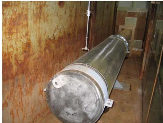
Figure 1. WTEV75 Cylindrical screen inside test flume.
