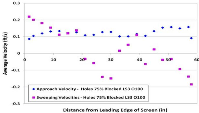
**Figure 5.** Approach and sweeping velocities measured 3 inches from the screen along the left side (LS3) – WTEV75 configuration.
