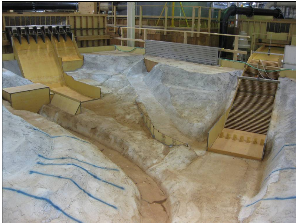
Figure 5. 1:48-scale physical hydraulic model of the main Folsom Dam, auxiliary spillway, and confluence area where flows combine in the American River.
