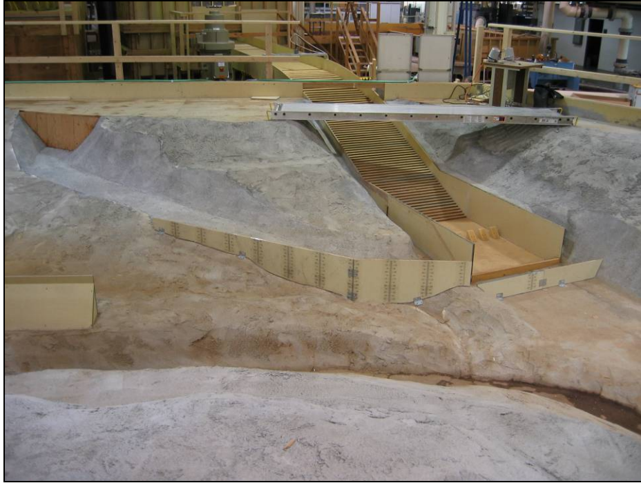
Figure 6. Installation of plywood cofferdam sections in the model. Model topography was modified to incorporate the construction access road.
