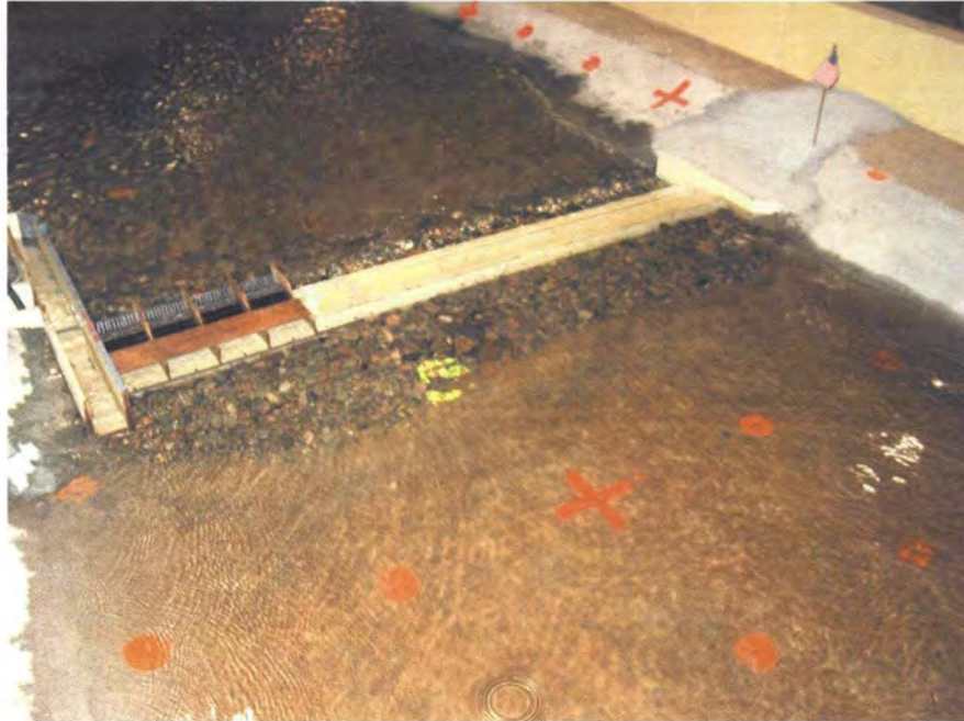
Figure 21. - Overall view of flow over the barrier with Q=5000 \text{ ft}^3/\text{s} and the gates up.
