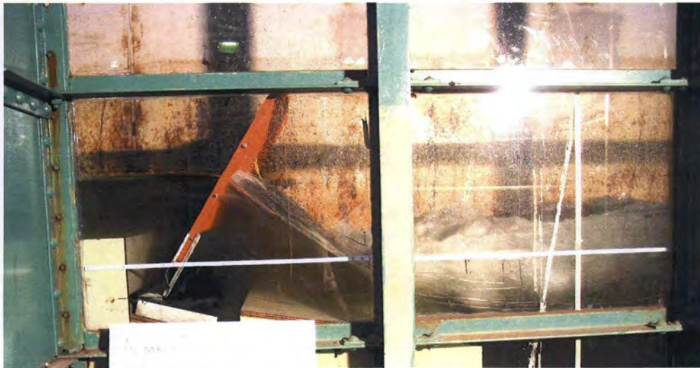
Figure 6. - Flow conditions for Q=7000 \text{ ft}^3/\text{s} , TW=\text{El. } 80.02 \text{ ft} through the sectional model of the picketed gate. Note the flow depth and location of the jump relative to the gate and the sill.
