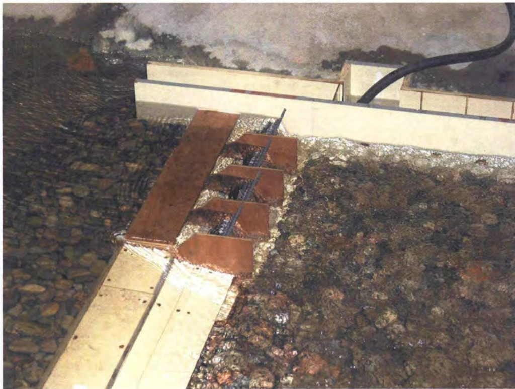
Figure 22. - View of the area adjacent to the ladder with Q=5000 \text{ ft}^3/\text{s} over the entire structure and the gates up.
