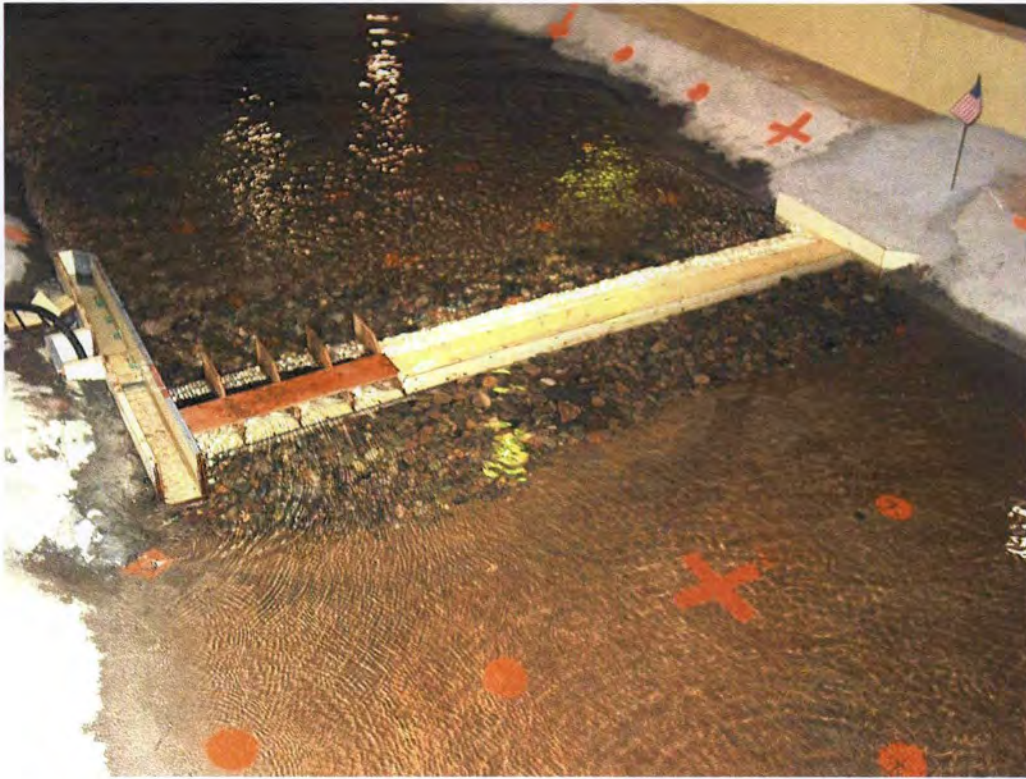
Figure 15. - Overall view of the barrier with Q=5000 \text{ ft}^3/\text{s} and the bypass gates down. Flow is over the sill and fairly uniformly distributed across the river.
