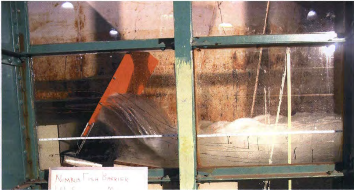
Figure 5. - Flow conditions for Q=5000 \text{ ft}^3/\text{s} , TW=\text{El. } 79.03 \text{ ft} through the sectional model of the picketed gate. Note the flow depth and location of the jump relative to the gate and the sill.
