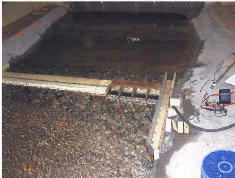
Figure 16. - Looking upstream at the bypass and ladder entrance area with Q=5000 \text{ ft}^3/\text{s} . Flow is from the top to the bottom in the photo.
