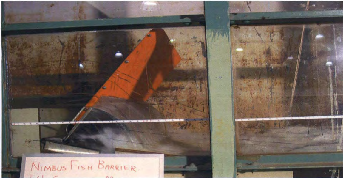
Figure 3 - Flow conditions for Q=1500 \text{ ft}^3/\text{s} , TW=\text{El. } 76.5 \text{ ft} through the sectional model of the picketed gate. Note the flow depth and location of the jump relative to the gate and the sill.
