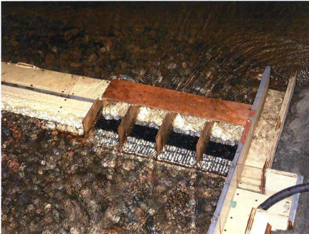
Figure 18. - View of the bypass and entrance area with Q=7000 \text{ ft}^3/\text{s} and the gates down. Flow is from top to bottom.
