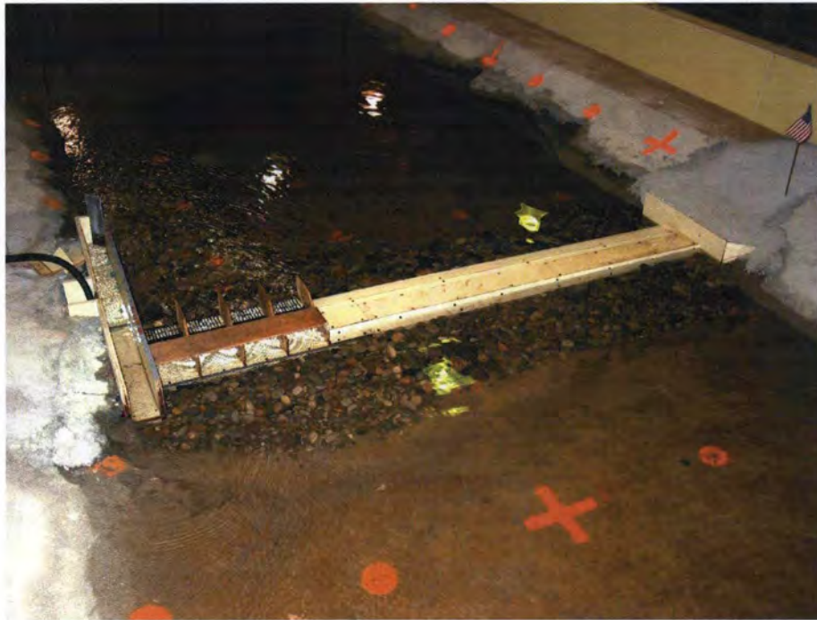
Figure 13. Overall view of the barrier with Q=1500 \text{ ft}^3/\text{s} and the gates down. Flow is only going through the bypass.
