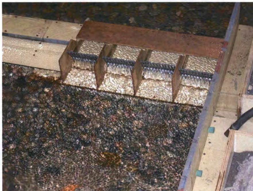
Figure 20. – Looking upstream at the bypass and ladder entrance area with Q = 1500 \text{ ft}^3/\text{s} . Flow is from the top to the bottom in the photo.
