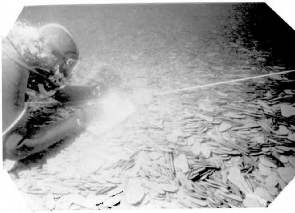
Figure 2. - Platelet type of erosion from bedded clay transported 366 mm (1200 ft). Project photograph by T. J. Spicher.
