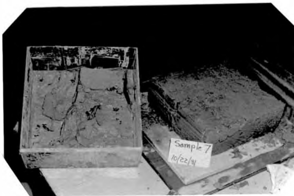
Figure 11. - Layer of mushy clay stuck to bottom of plastic handling box.
