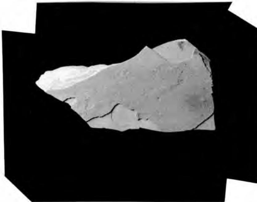
(b) Underside of same piece showing thin lamina of leaner sandy clay adjacent to fatter clay lamina.
