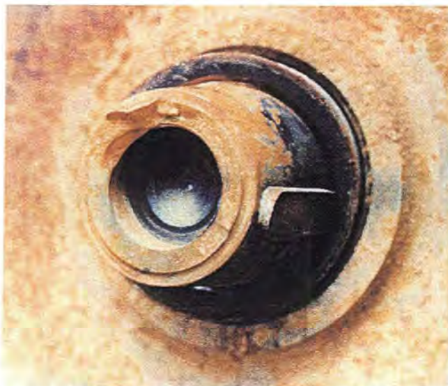
Figure 26. Broken shaft on Wemco pump. First occurrence of broken shaft, likely due to fatigue damage.
