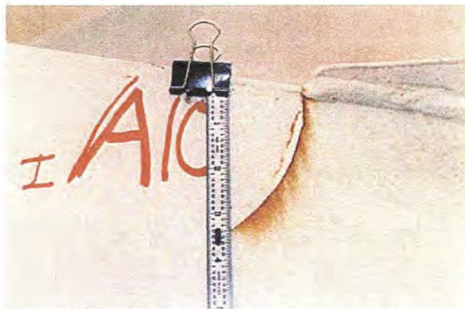
Figure 21. Typical fatigue crack propagation. Cracking generally propagated perpendicularly from the edge of the weld. Note the abrupt material transition at the weld, responsible for stress concentration.
