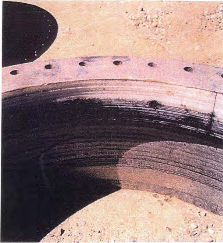
Figure 14. UHMW seal ring. Wear and scoring on UHMW seal ring on Archimedes pumps, due to sediment intrusion.
