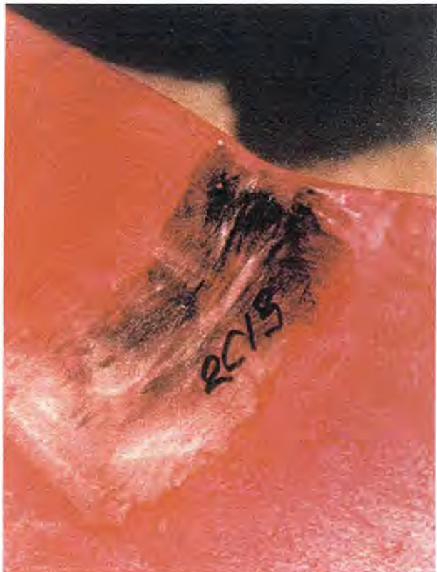
Figure 22. Weld repair to Archimedes flights. Weld repair on cracked flight. Note contoured joint at plate interface.
