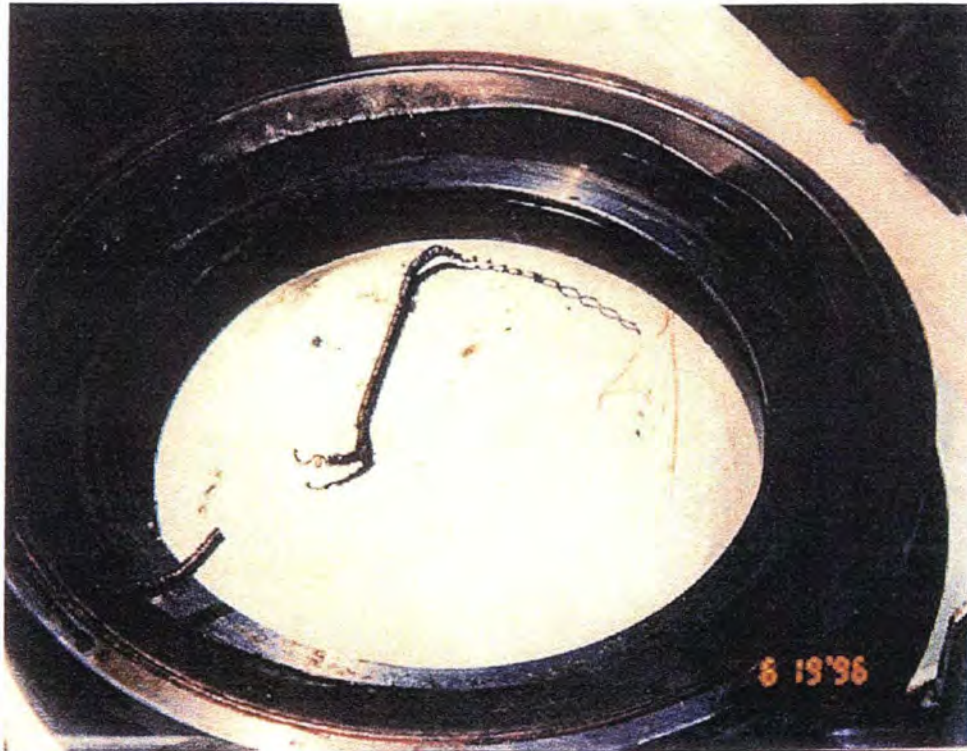
Figure 17. Damaged seal ring from thrust bearing. Damaged seal ring, note broken spring and pry marks on steel shell.
