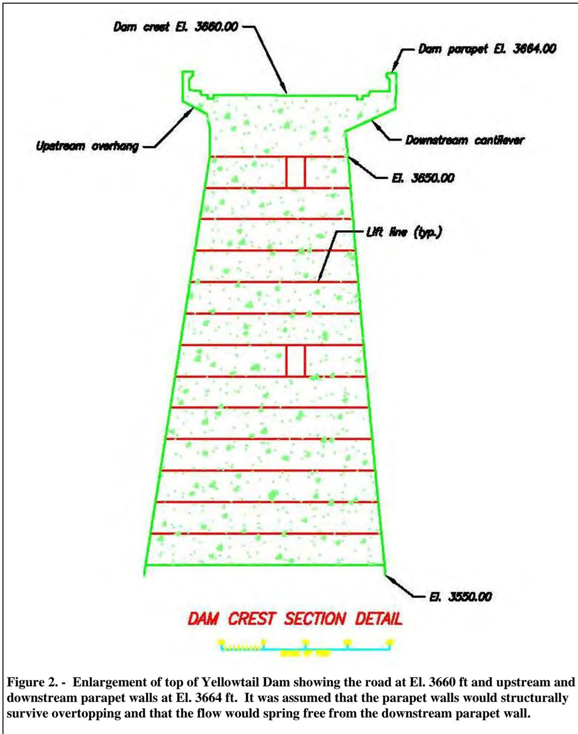
Figure 2. - Enlargement of top of Yellowtail Dam showing the road at El. 3660 ft and upstream and downstream parapet walls at El. 3664 ft. It was assumed that the parapet walls would structurally survive overtopping and that the flow would spring free from the downstream parapet wall.
