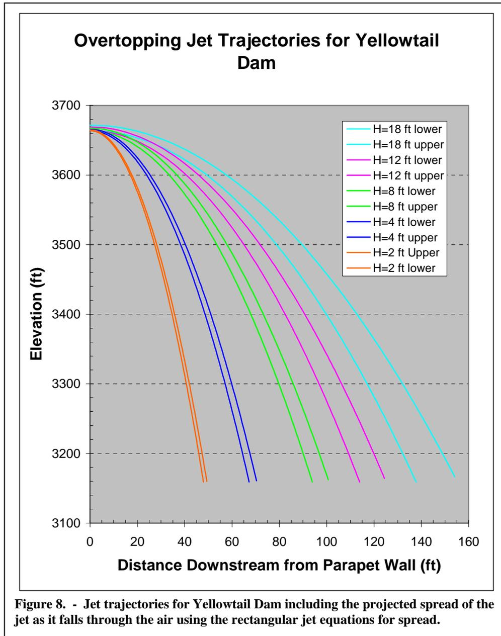
Figure 8. - Jet trajectories for Yellowtail Dam including the projected spread of the jet as it falls through the air using the rectangular jet equations for spread.
