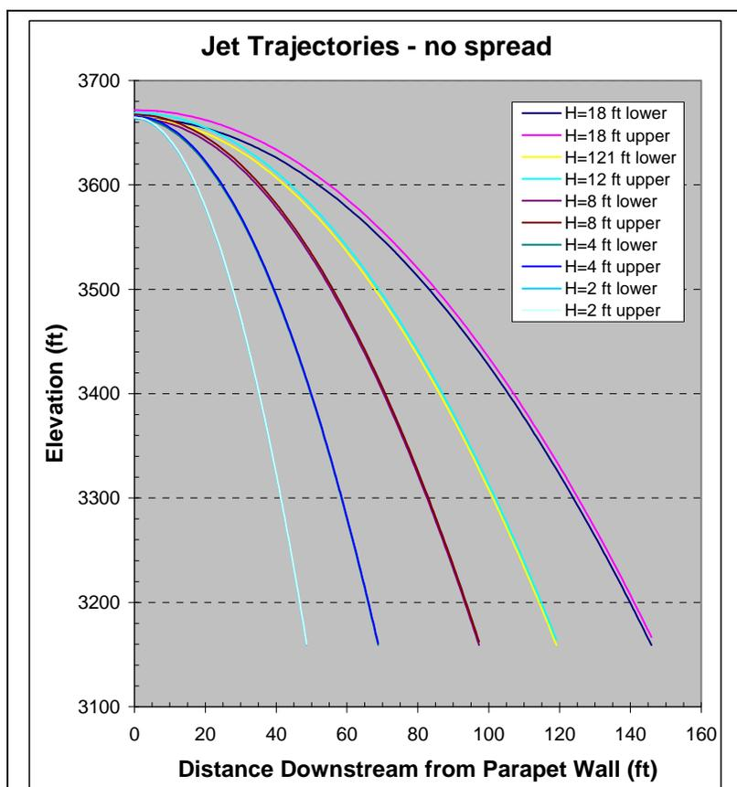
**Figure 6. - Sectional view of the trajectory profiles, with equations of motion only, for the overtopping head range investigated for Yellowtail Dam. (Note the trajectories all originate at the downstream parapet wall on the top of the dam road.)**
