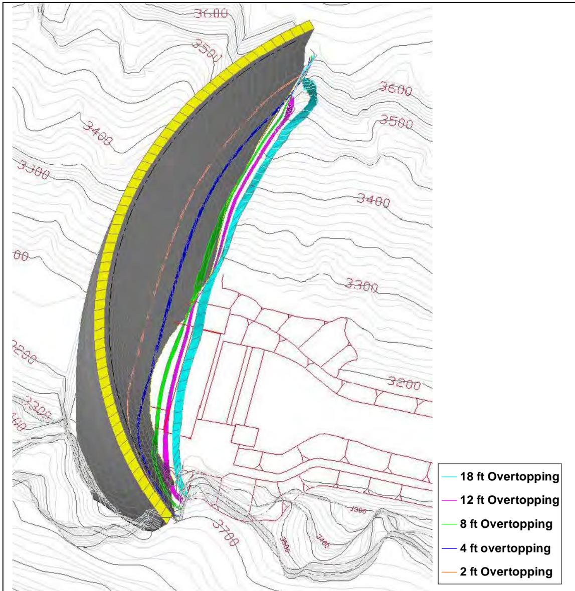
**Figure 10. - Isometric view of the trajectories impingement locations for the overtopping events of 2, 4, 8, 12 and 18 ft of head for Yellowtail Dam.**
