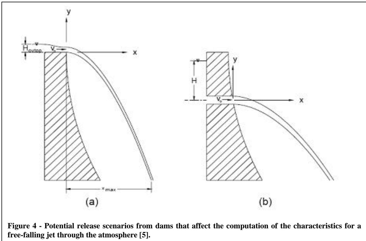
Figure 4 - Potential release scenarios from dams that affect the computation of the characteristics for a free-falling jet through the atmosphere [5].
