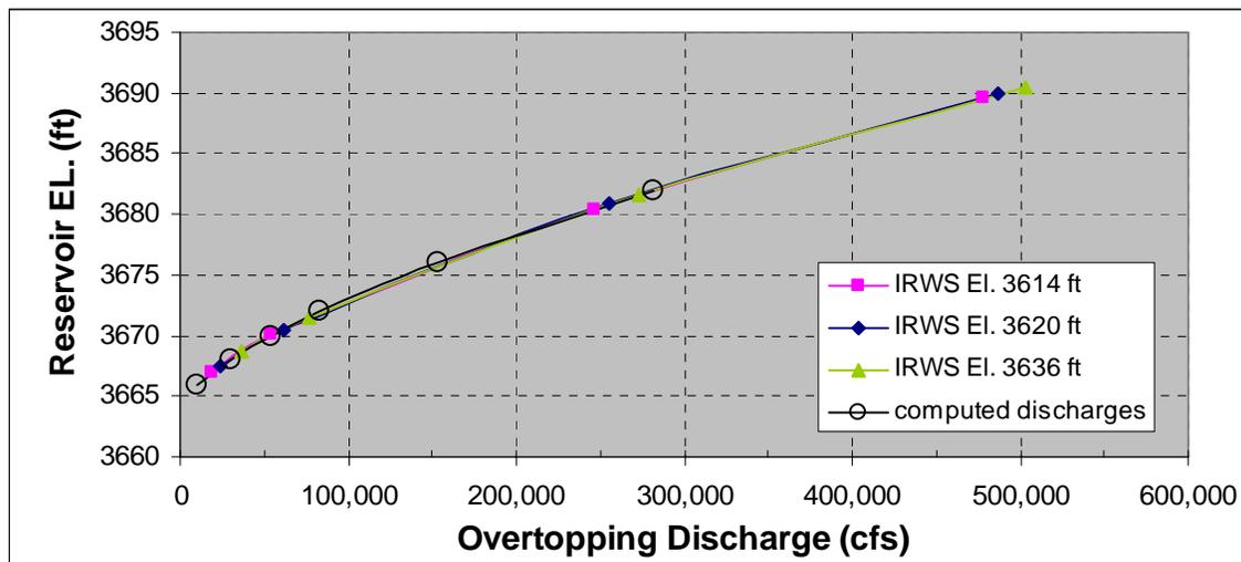
**Figure 3. - Discharges overtopping the parapet wall at Yellowtail Dam created during flood routings and computed for the requested reservoir overtopping heads [16].**
