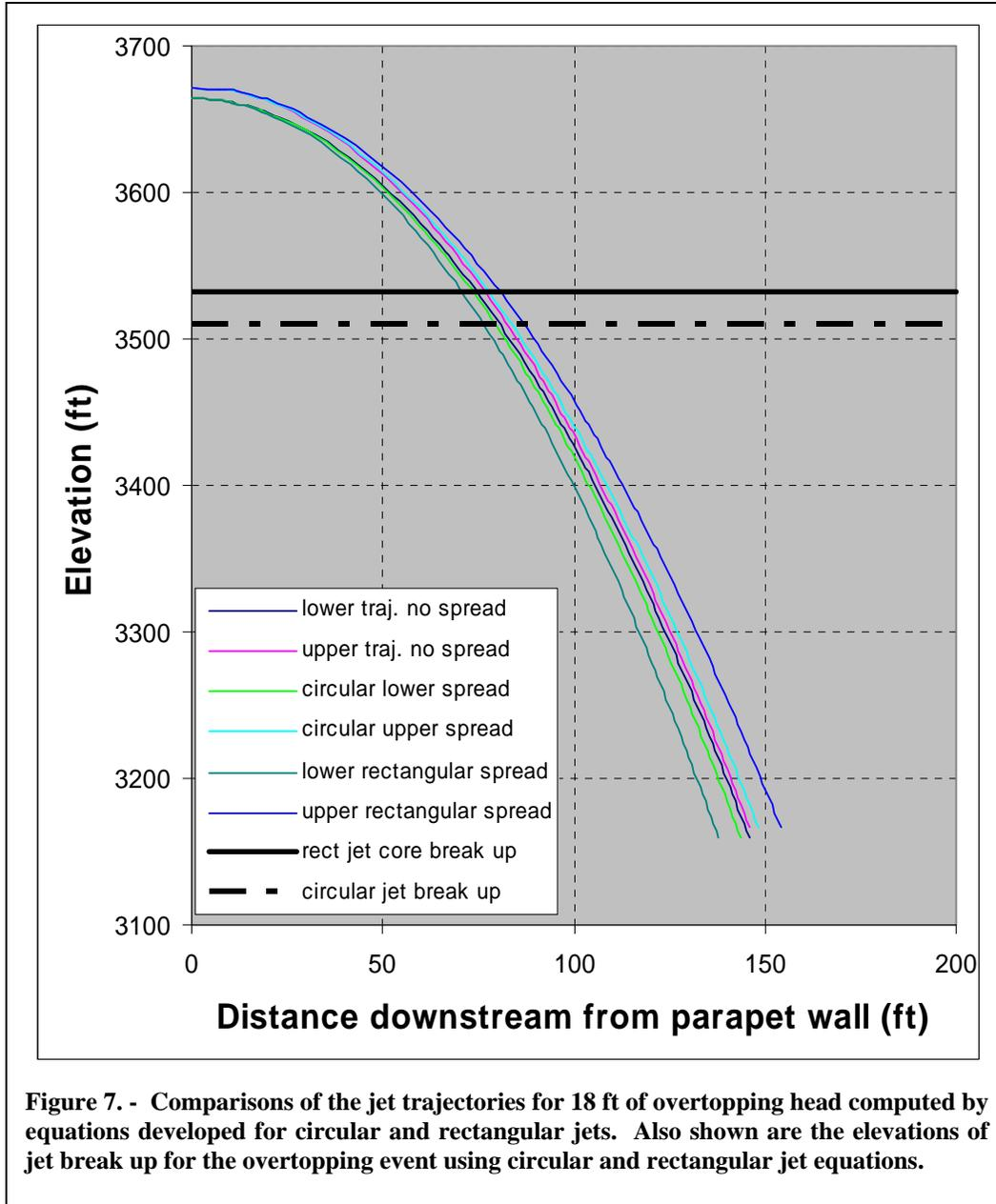
Figure 7. - Comparisons of the jet trajectories for 18 ft of overtopping head computed by equations developed for circular and rectangular jets. Also shown are the elevations of jet break up for the overtopping event using circular and rectangular jet equations.
