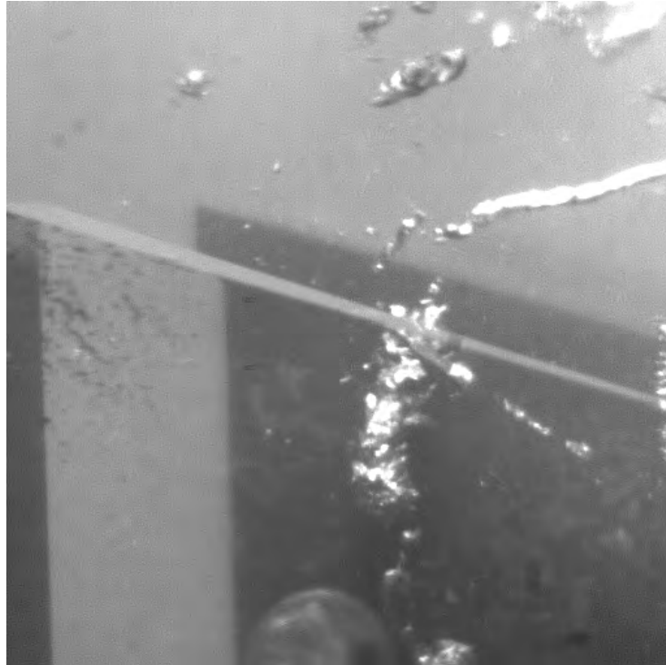
Figure 5: Near vertically oriented vortices in the shear layer between blocks. Half block against wall in clear acrylic to facilitate viewing between the blocks.
