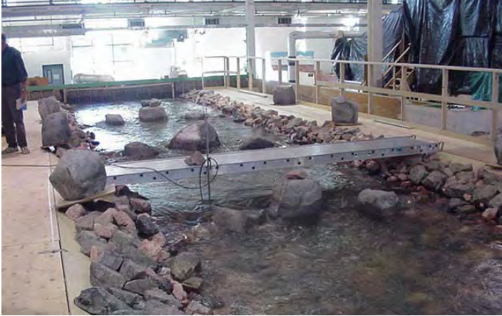
Figure 2 – View of a full scale roughened-channel test facility used to study non-salmonid passage using chevron shaped boulder weir drops.
