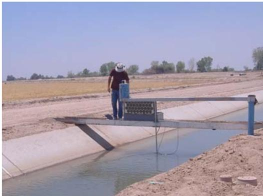
Figure 9. ADFM unit at Potter Flume
