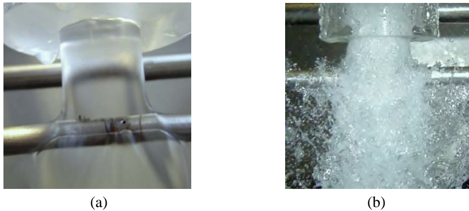
Figure 3 – Combined probe testing: (a) clear-water flow; (b) air-water mixture.
