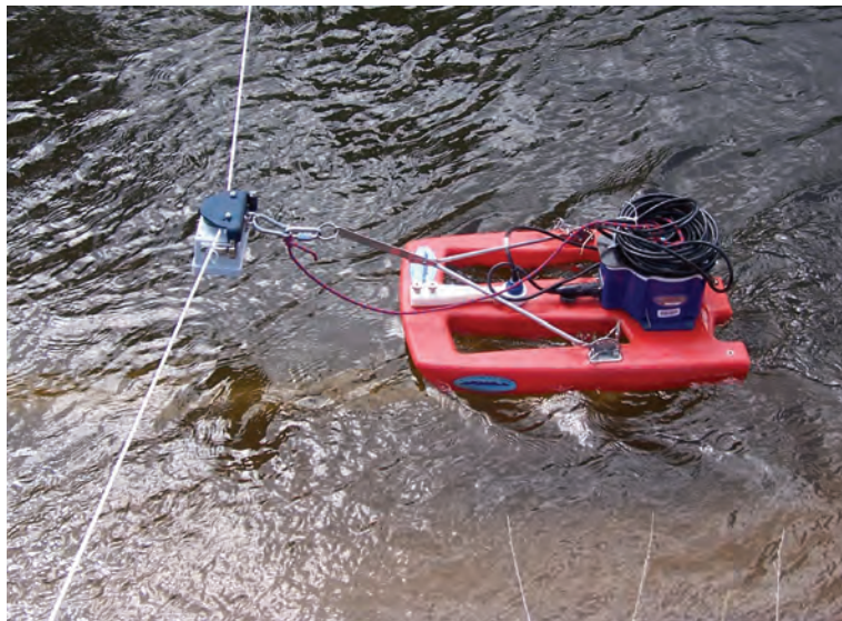
Figure 2: StreamPro deployed on a tagline with an Ocean Science Cable Chimp (radio controlled cableway ROV) for taking moving boat discharge measurements.
