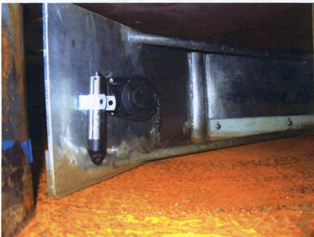
Figure 8 - View of pressure logger mounted on a vane of the rotary valve.
