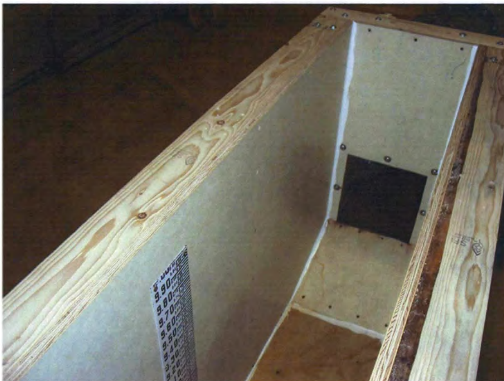
Figure 7 - View of entrance flume constructed for the laboratory evaluation.
