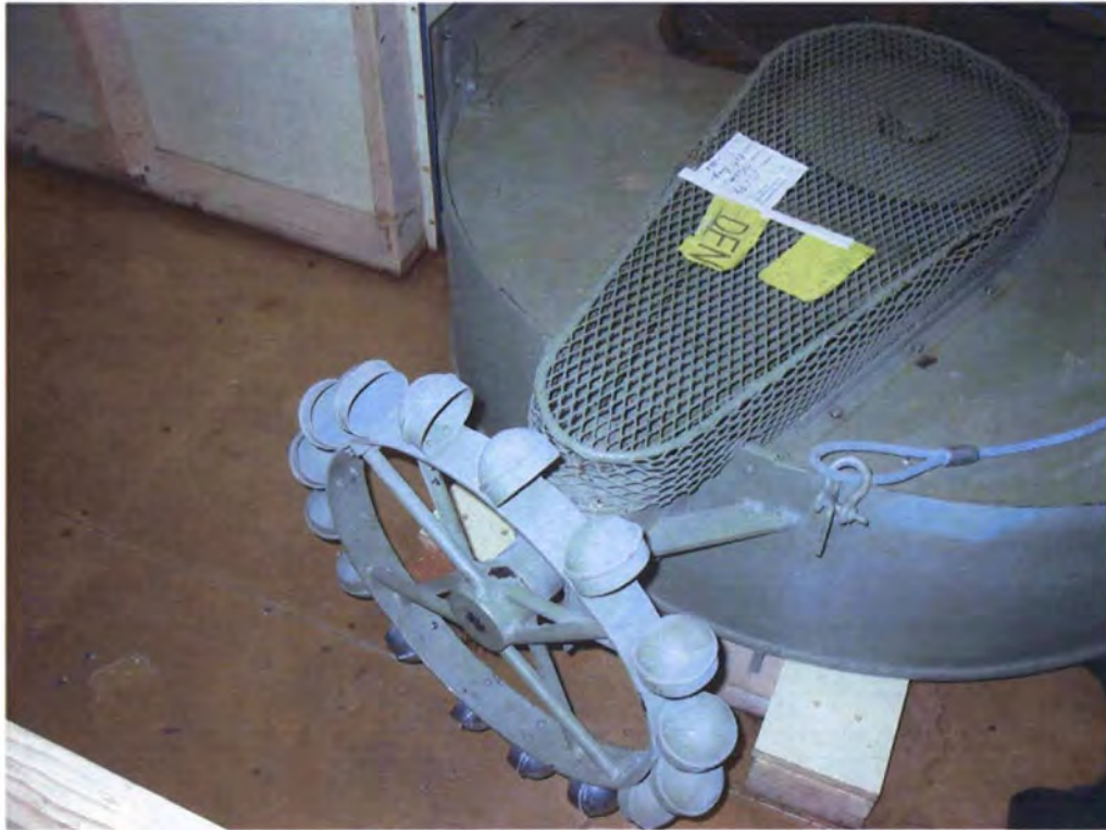
Figure 3 - View of overshoot water wheel.
