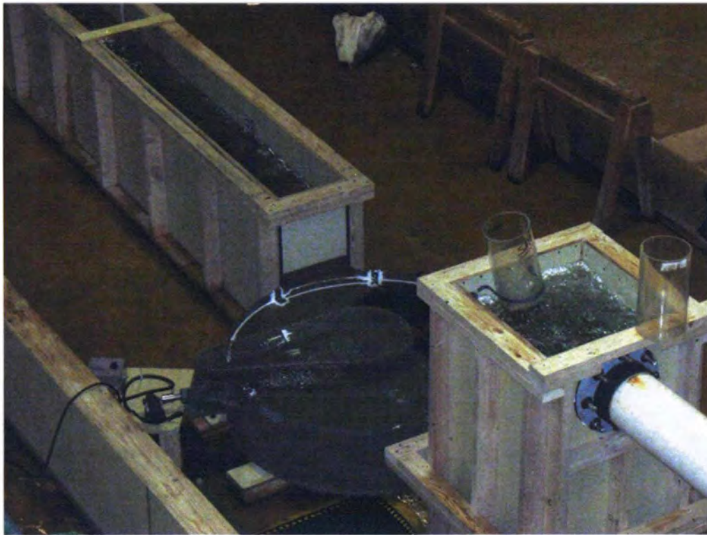
Photograph 3– View of model showing wet well at the upstream exit of the rotary valve. Plastic tubes shown on at the surface of the wet well were used to view fish exiting the valve.
