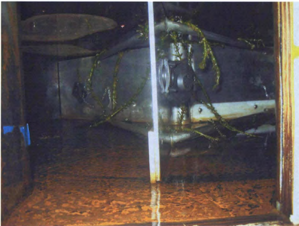
Figure 17 – View looking in side rotary valve directly at a vane following tests of aquatic pond weed entrapment.
