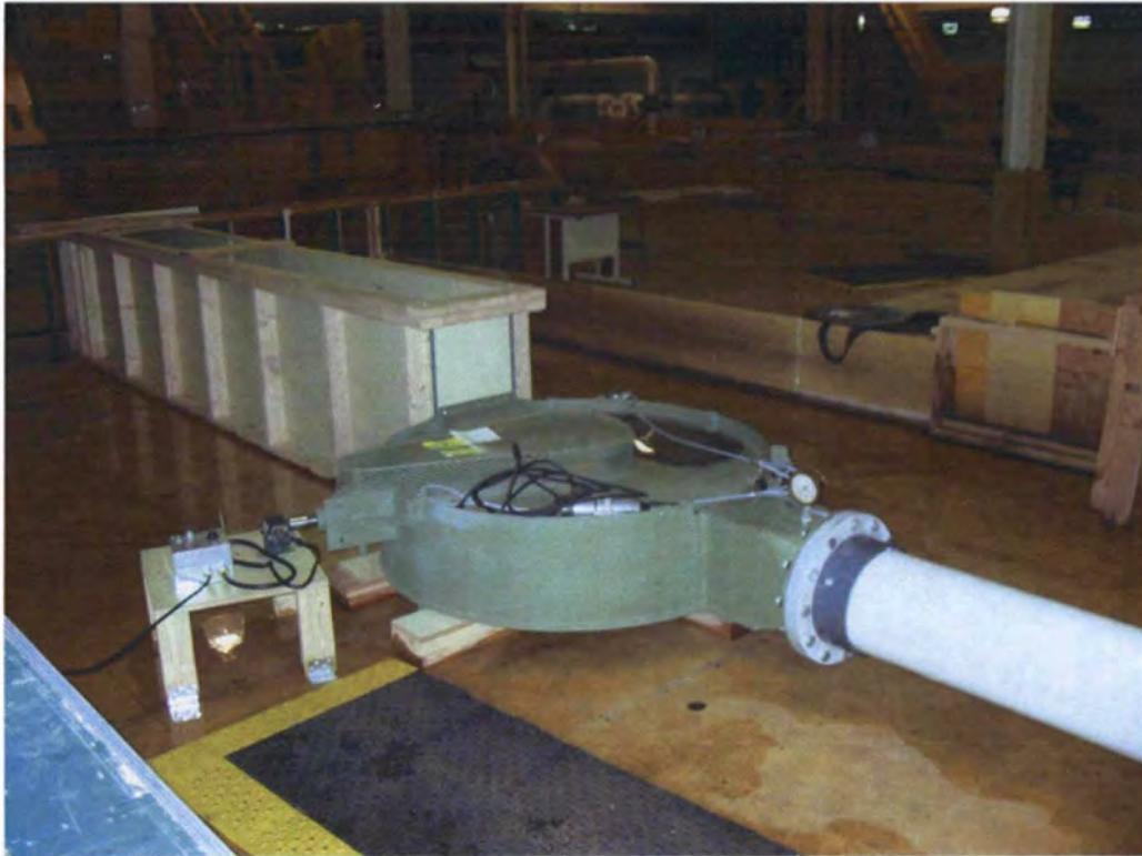
Figure 5 - View of test setup with a downstream flume and an upstream pipe from a pump. (Flow passes through from right to left)
